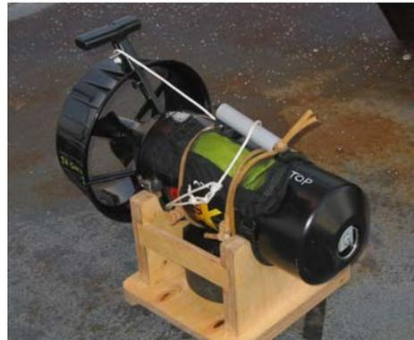
*Figure 6: X-Scooter diver delivery vehicle*
