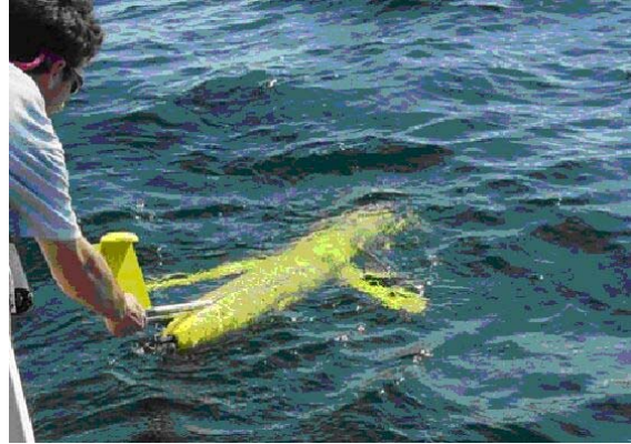
Figure 5: Slocum Glider being released.
