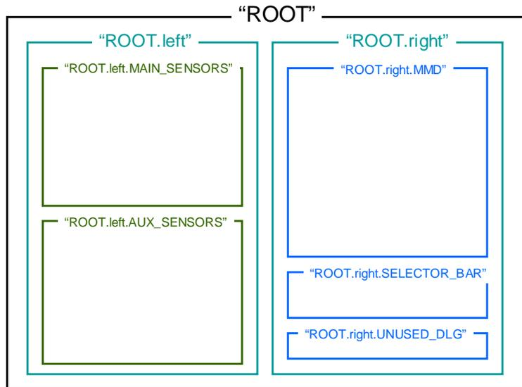
**Figure 7. Example of hierarchical subdivision of Operator View**
