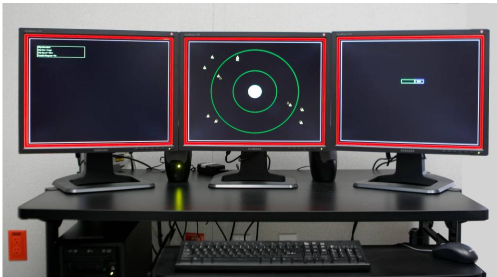
Figure 5. Screen capture of the Flashing border alert displayed on all three screens.
