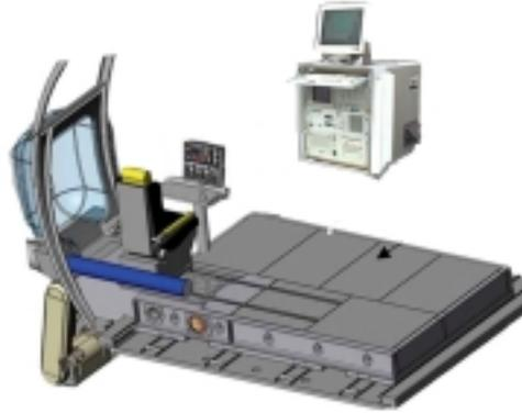
**Figure 17. RMAS Palette with the AS-7 strut that will hold the Radar Antenna Pod. Radar Rack is shown to scale. The addition of a real time processor increases the equipment size by 50%.**
