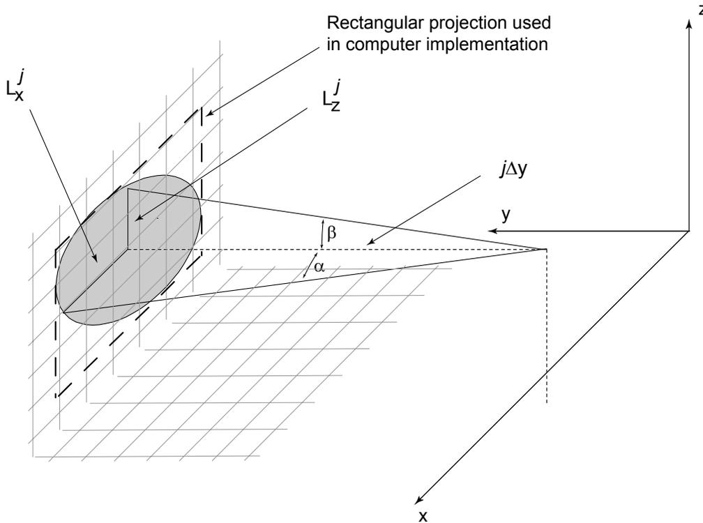
**Figure 15.** Projection of beam in 3D coordinate system.
