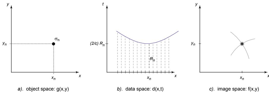
**Figure 1.** Coordinate systems used in synthetic aperture imaging.
