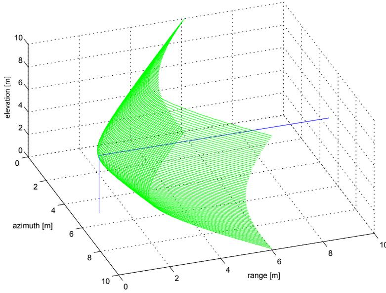
**Figure 6.** PSR surface for extended vertical array.
