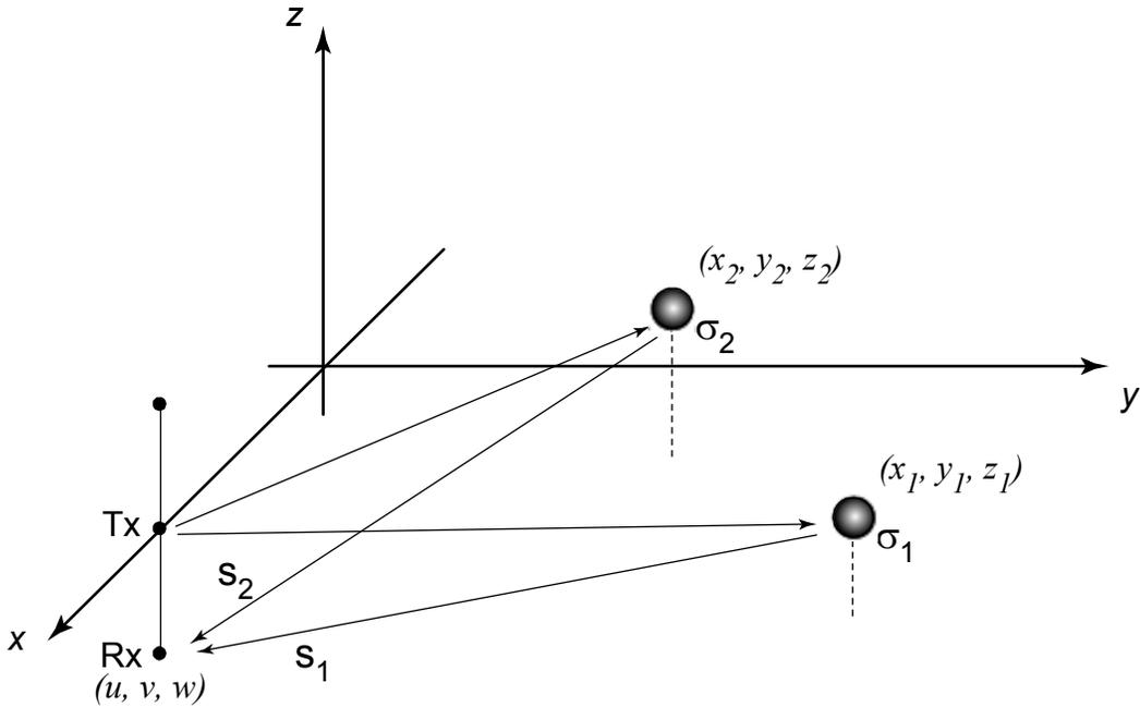
**Figure 3.** Composite signal received at array elements.
