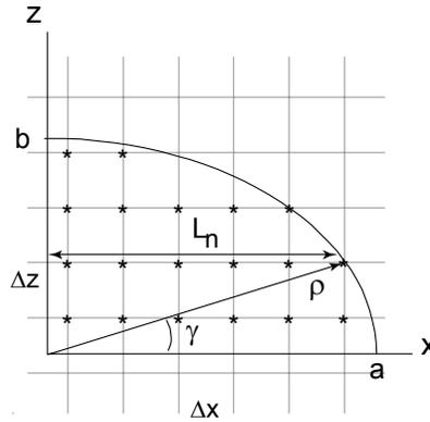
**Figure 16.** Interpolation of grid points for elliptic projection.
