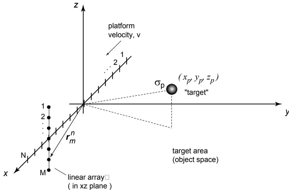
Figure 2. 3D imaging geometry.
