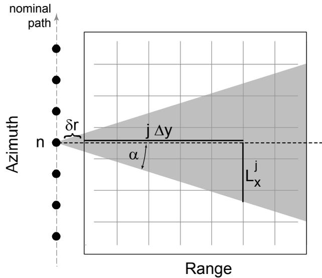
Figure 12. Parameters used in finite beamwidth processing.
