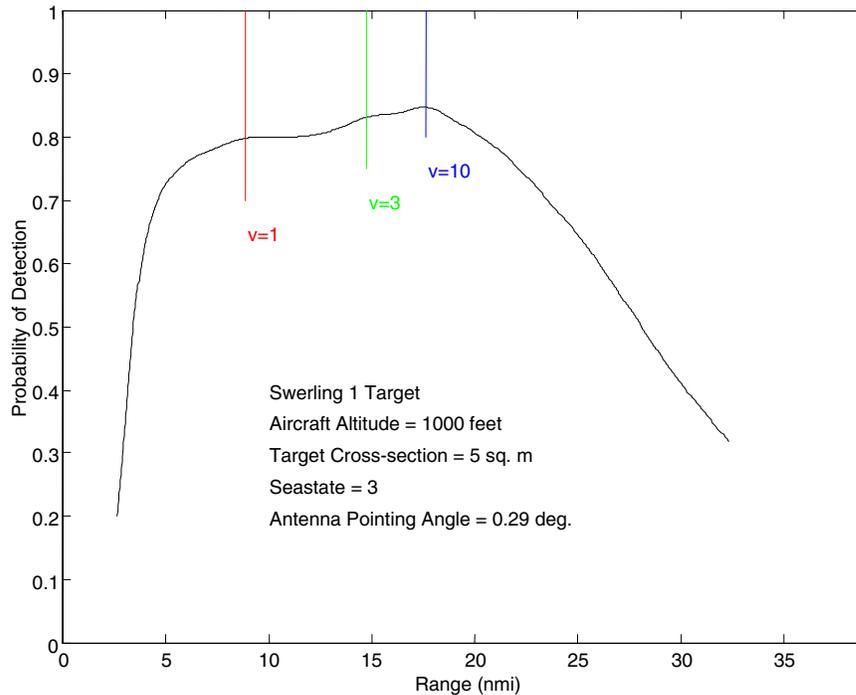
**Figure 5.** Probability of detection versus range for 5 m<sup>2</sup> Swerling 1 target from aircraft altitude of 1000 feet with Douglas sea state 3. Range locations at which underlying K distribution shape parameter equals 1 (red), 3 (green) and 10 (blue) are indicated.
