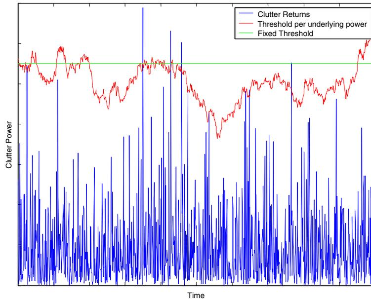
**Figure 1. Fixed and variable threshold settings to achieve equivalent PFA.**
