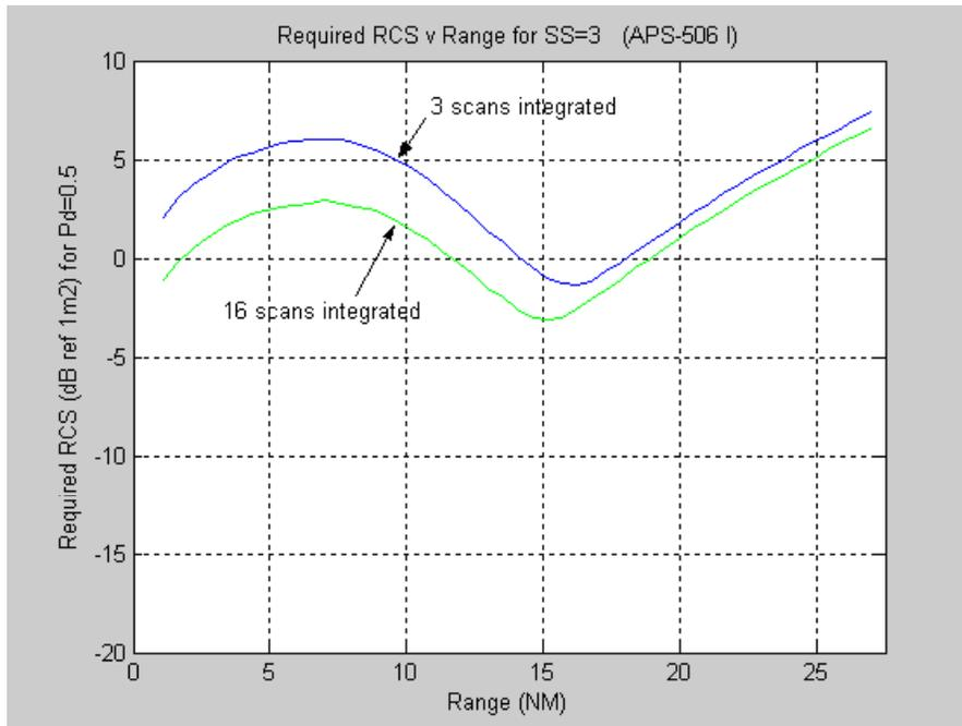
**Figure 2. Required RCS for 50% probability of detection in Sea State 3 with assumption of integration of 3 and 16 independent scans.**
