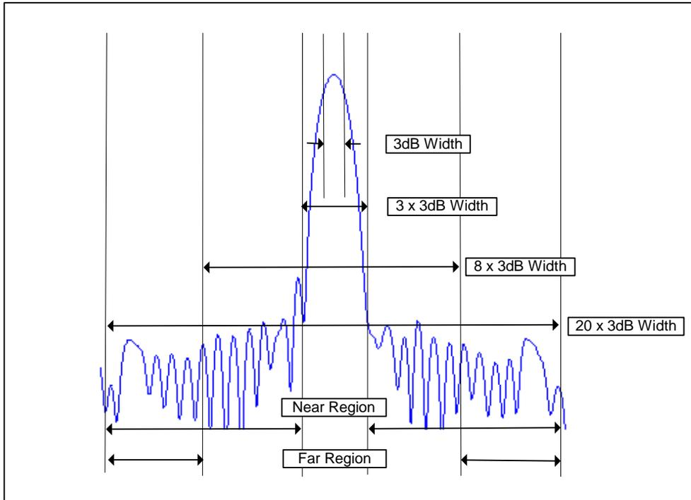
**Figure 7. Impulse response: Near and far region specifications.**
