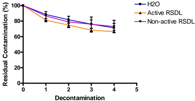
Figure 12: Residual contamination levels of <sup>99m</sup>Tc after decontamination attempts using Active or Non-active RSDL.
