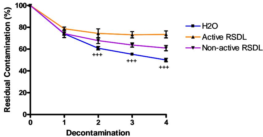
Figure 10: Residual contamination levels of <sup>64</sup>Cu after decontamination attempts using Active RSDL or Non-active RSDL.
