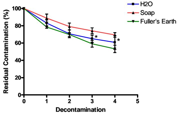
Figure 11: Residual contamination levels of <sup>99m</sup>Tc after decontamination attempts using water, soap, or Fuller's Earth.
