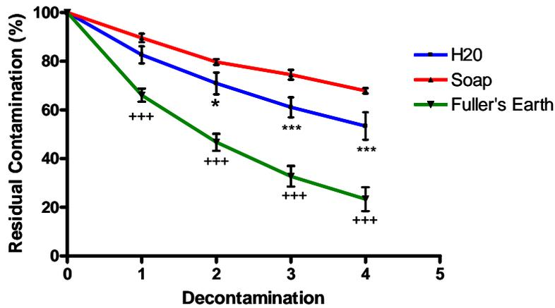
Figure 7: Residual contamination levels of <sup>42</sup>K after decontamination attempts using Water, Soap or Fuller's Earth paste.
