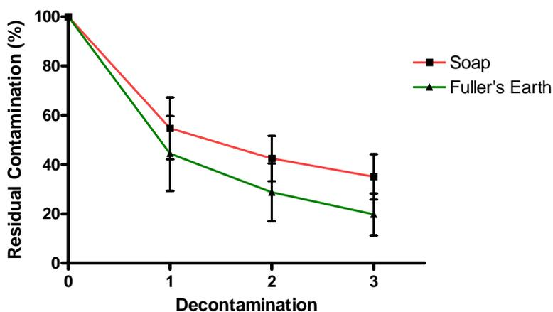
Figure 6:  $^{24}\text{Na}$  decontamination with Soap or Fuller's Earth paste.
