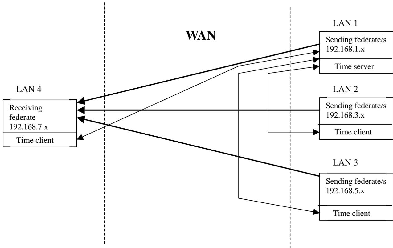
Figure 2-2 Experimental Network Setup
