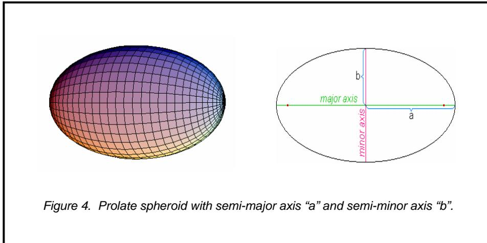
In this case, we assume that the ship can be modeled as a single prolate spheroid with permanent magnetization  $\mathbf{M}_P$  and induced magnetization  $\mathbf{M}_I$ , both in Ampere/metre. The permanent magnetization has the components  $(M_{Px}, M_{Py}, M_{Pz})$ , and the induced magnetization is a function of the geometry of the prolate spheroid and the magnetic susceptibility  $\chi_m$ , a dimensionless parameter given by (Ref 5, pages 172-173):
