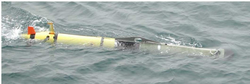
Figure 1. The NSW-PC REMUS autonomous underwater vehicle.
