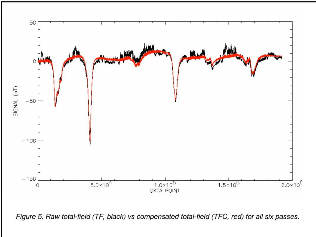
Figure 5. Raw total-field (TF, black) vs compensated total-field (TFC, red) for all six passes.
