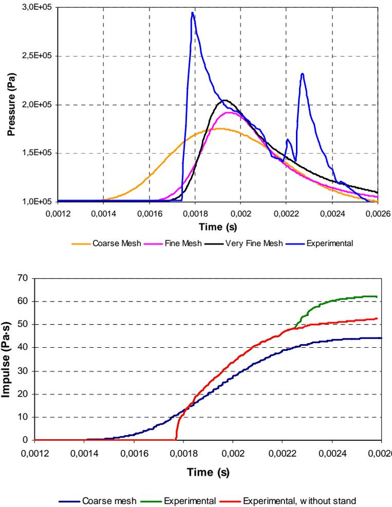
Figure 5: Pressure and impulse profiles for different mesh and from experiments (1 lb of C4 with stand)
