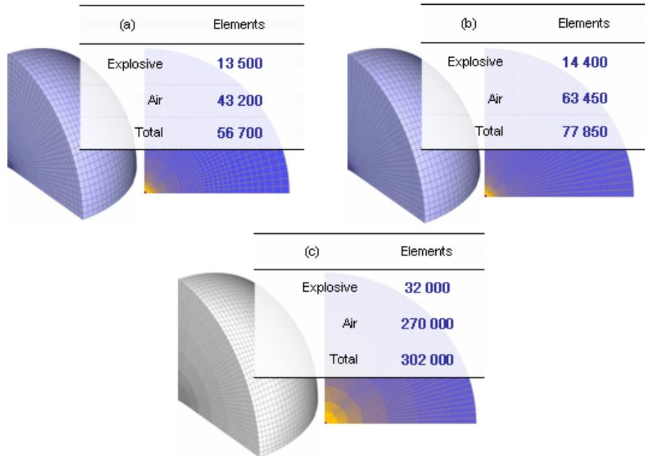
Figure 4: Total elements in coarse mesh (a), fine mesh (b) and very fine mesh (c)
