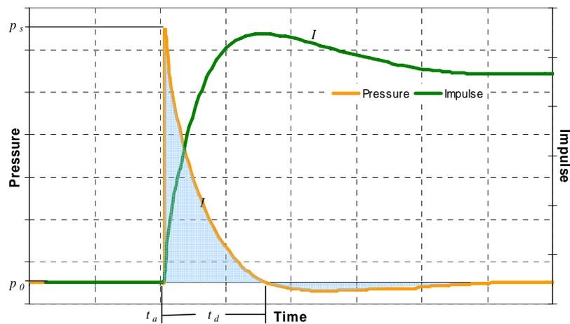
Figure 1: The typical pressure versus time curve at a stationary point
