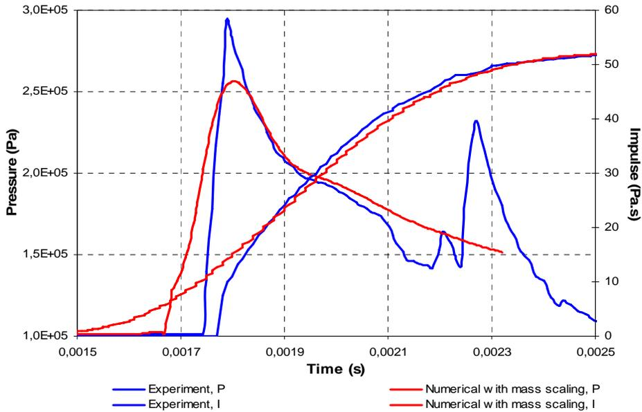
Figure 8: Comparison between experimental and the numerical pressure and impulse profile using a mass-scaling factor
