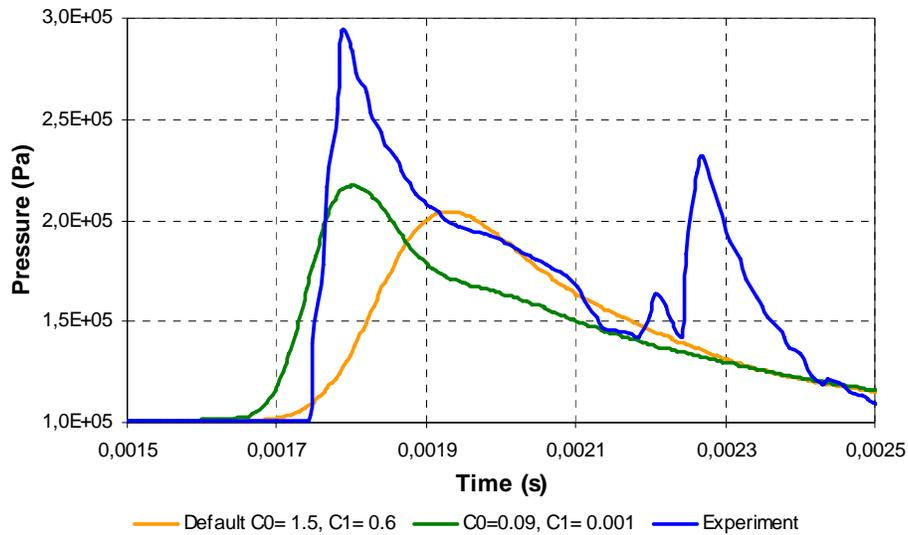
Figure 7: Comparison between experimental data and two different bulk viscosity values: the LS-DYNA default and the one used in this study
