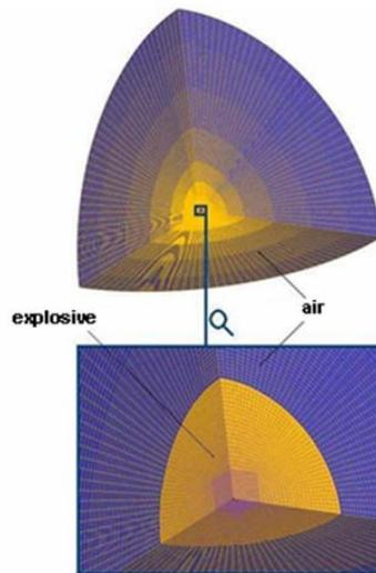
*Figure 2: Finite element model with coarse mesh*
