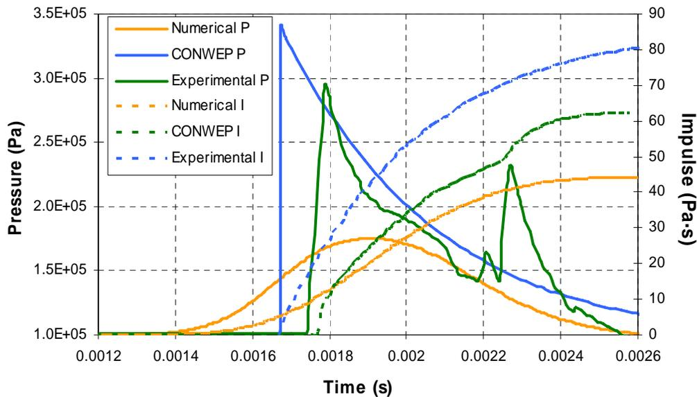
Figure 3: Comparison of numerical results (coarse mesh) with CONWEP and experimental data from Ref. 3 (1 lb C4). In the legend, P means pressure and I the impulse
