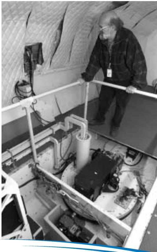
*Ground Moving Target Indication (GMTI) radar equipment.*
