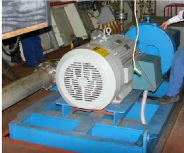
*Figure A-7. Shadwell High-Pressure Water Mist Pump*
