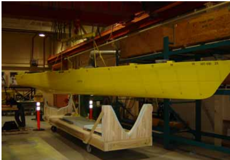
Figure 5: 1:13.54 Scale HALIFAX Class Frigate Model
