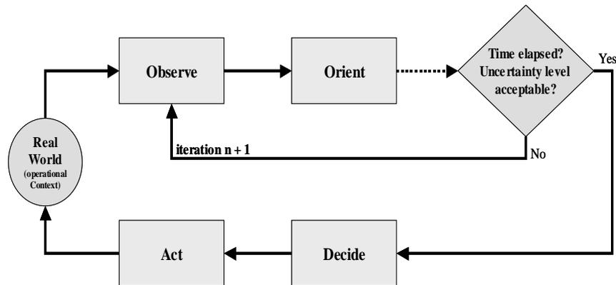
Figure 3: The iterative version of the OODA loop [11]
