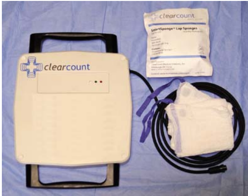
Figure 16: Wand scanner (left) and RFID-tagged sponges [51].
