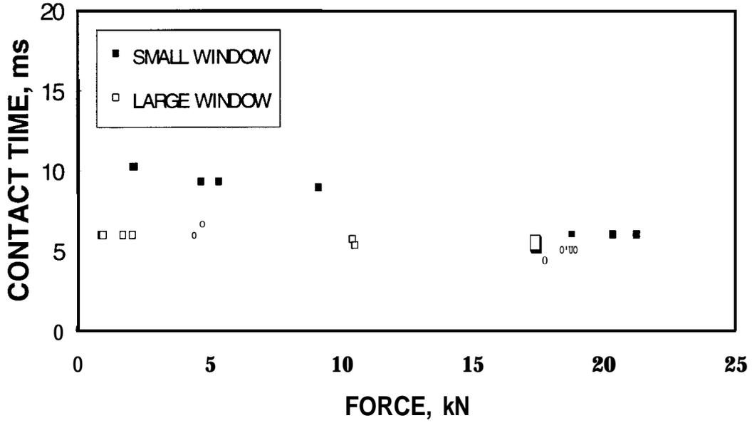
Figure 3 Contact Time of the Sledge Hammer for Impacts on the Small and Large Windows at Location U
