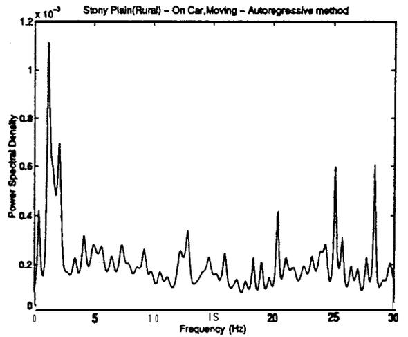
Fig. 5 Vibration: Power spectra of police vehicle during highway patrol
