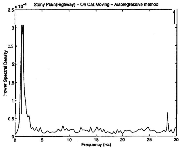
**Fig. 6 Vibration: Power spectra of vibration on police officers in police vehicle during municipal policing**
