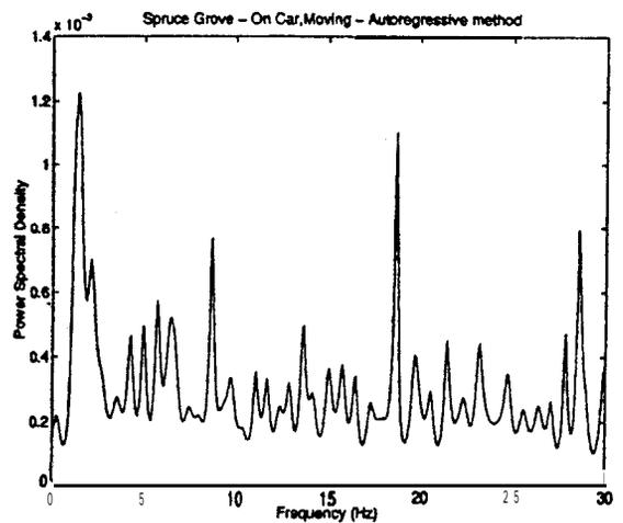
Fig. 4 Vibration: Power spectra of police vehicle in rural policing
