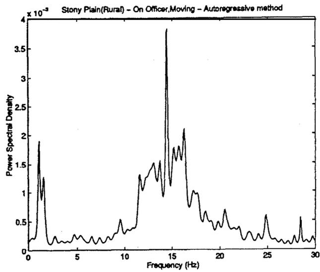
**Fig. 8 Vibration: Power spectra of vibration on police officers in police vehicle during highway patrol**
