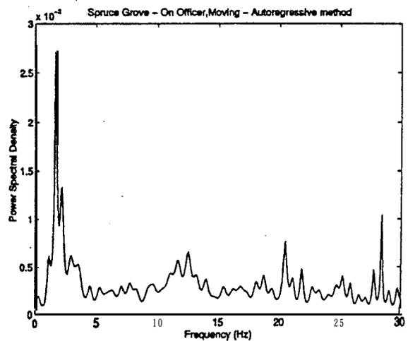
**Fig. 7 Vibration: Power spectra of vibration on police officers in police vehicle during rural policing**
