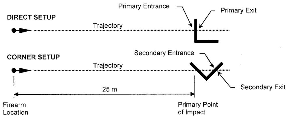
Figure 2 - Test Setup for "Direct" and "Corner" Shots
