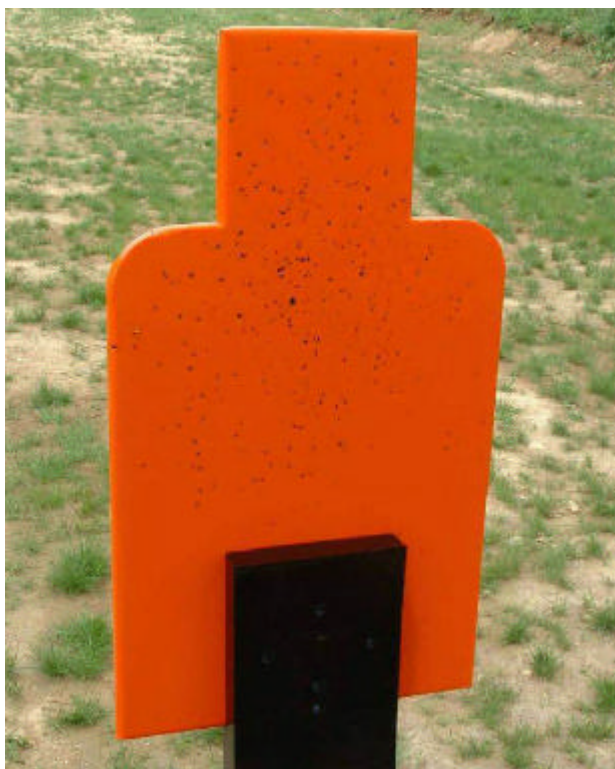
Figure 2.2: Alternative Target Type 2: M-T36 Ballistic Polymer Unit
