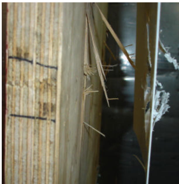
Figure 4.3: Typical failure of Original Warning Shot Target, Post Impact Side view
