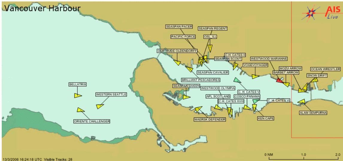
Figure 4. The positions of AIS-equipped vessels in Vancouver harbour on March 13<sup>th</sup>, 2006 are shown using isosceles triangles labelled with the vessel name.<sup>12</sup>
