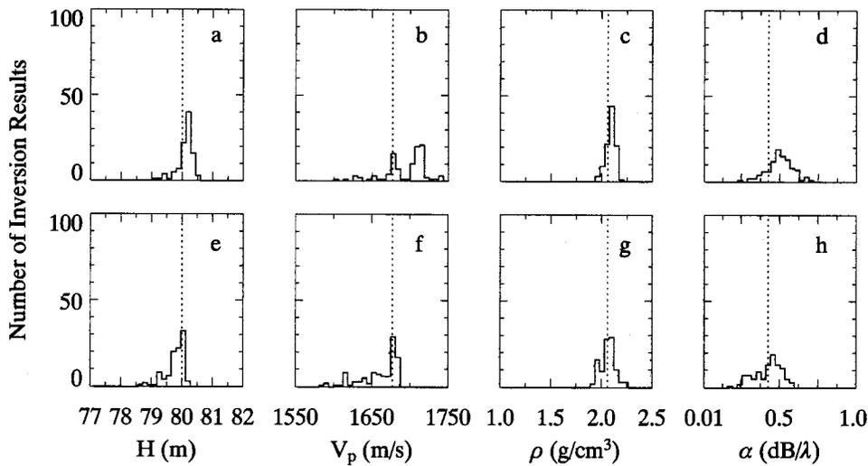
FIG. 10. Comparing different ranges. The histograms of the inversion results for studies V4 ( $R=15$  km) shown in (a)–(d) and V2 ( $R=4$  km) shown in (e)–(h) are presented. The inversion results include model parameter values for  $H$ ,  $V_p$ ,  $\rho$ , and  $\alpha$ . The vertical lines and abscissa limits are as described in Fig. 6.
