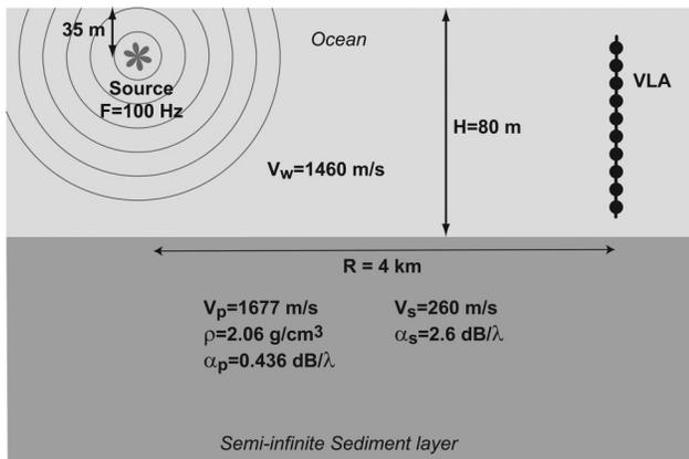
FIG. 1. Schematic representation of the basic ocean environment and “experimental setup” used for this study, including source frequency  $F$ , water sound speed  $V_w$ , water depth  $H$ , range  $R$ , sediment compressional speed  $V_p$ , sediment density  $\rho$ , compressional wave attenuation  $\alpha_p$ , shear speed  $V_s$ , and shear attenuation  $\alpha_s$ .
