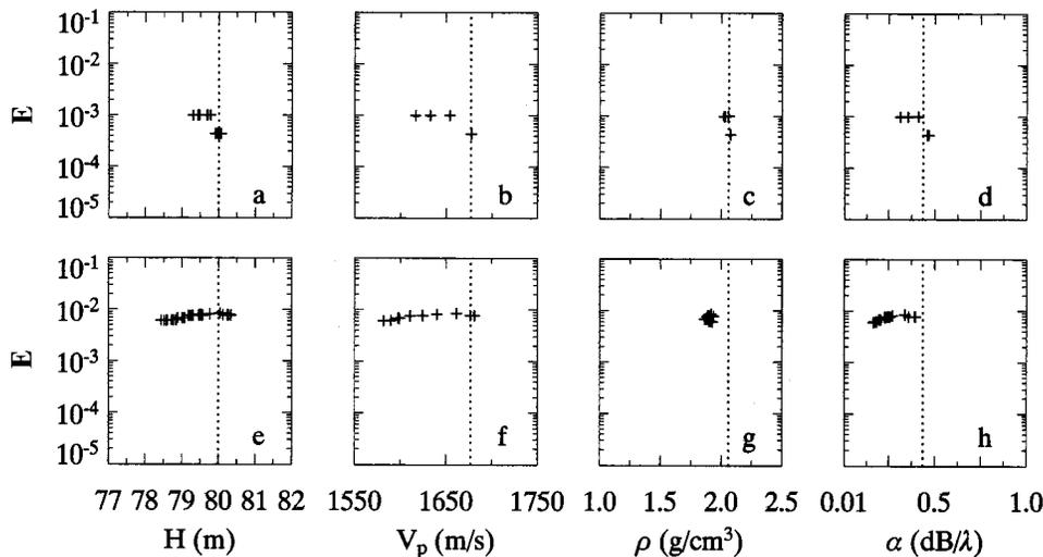
FIG. 5. Mismatch vs model parameter values for inversion solutions for studies V2(a) shown in (a)–(d) and V2(b) shown in (e)–(h) are presented ( $s_{vx} = \pm 20$  m/s). For each study, a unique range-dependent environment was used. The model parameters, abscissa limits, and vertical dotted lines are as described in Fig. 3.
