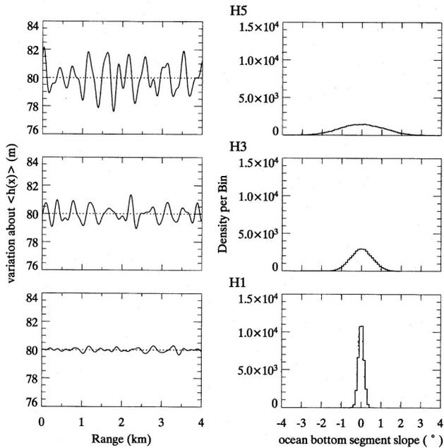
FIG. 13. Variable water depth. Sample realizations of the variable water depth are shown on the left-hand side for studies H1, H3, and H5. The dotted line represents the mean of the curve  $m_{hx}$ . On the right-hand side are histograms of all the slopes of the segments that make up each realization of the variable water depth used in the study.
