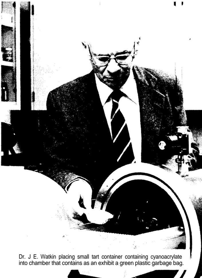
Dr. J. E. Watkin placing small tart container containing cyanoacrylate into chamber that contains as an exhibit a green plastic garbage bag.
