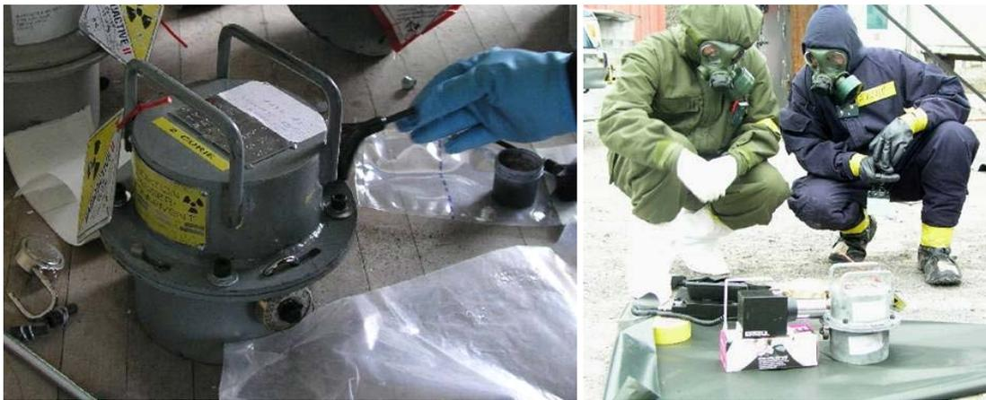
*Figure 3: Forensic (left) and radiological (right) analysis of pig containing seized Cs-137 source*
