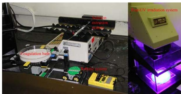
Fig. 1 Experimental set-up for fiber fabrication
