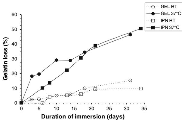
**Fig. 6** Stability through gelatin loss of the freeze-dried cross-linked gelatin (GEL) and gelatin-HydroThane™ IPN films, immersed in 0.1% sodium azide solution at room temperature (RT) and 37°C. Data are expressed as means ( $n = 2$ )
