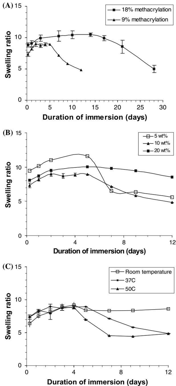
**Fig. 7** Effects of the methacrylation degree of gelatin (**A**), photoinitiator concentration (**B**) and incubation temperature (**C**) on rehydration and stability of the freeze-dried IPN films in a solution of 50% fetal bovine serum and 0.1% sodium azide. Data with error bars represent means  $\pm$  standard deviation ( $n = 3$ ), otherwise  $n = 1$ . The films were prepared using gelatin with 9% methacrylation
