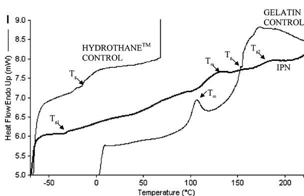
**Fig. 2** Typical DSC curves of crosslinked gelatin, HydroThane™ networks and gelatin-HydroThane™ IPN. The glass transition temperature,  $T_g$  is indicated by the corresponding arrow for the HydroThane™ control and the gelatin control. In the case of IPN, there are two glass transition temperatures,  $T_{g1}$  and  $T_{g2}$ . The glass transition temperatures were determined by the inflection points of each curve.  $T_m$  represents the melting temperature of gelatin
