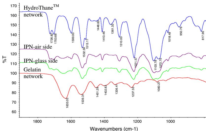
showed one peak at  $1633\text{ cm}^{-1}$  due to C=O and one peak at  $1539\text{ cm}^{-1}$  due to N-H. In the IPN spectrum, no new characteristic absorption bands and no significant shifts of these bands were noticed. Finally, Fig. 1 shows the IPN depicted relatively higher intensity of the urethane peaks on the side interfacing air during its preparation than on the side interfacing glass, implying more elastomer components due to higher surface tension on the airside.
