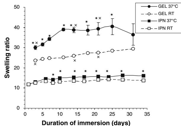
**Fig. 4** Rehydration characteristics of freeze-dried gelatin-HydroThane™ IPN and crosslinked gelatin (GEL) films immersed in a 0.1% sodium azide aqueous solution at room temperature (RT) and at 37 °C for up to 34 days. Values represent mean  $\pm$  standard deviation ( $n = 3$ )
