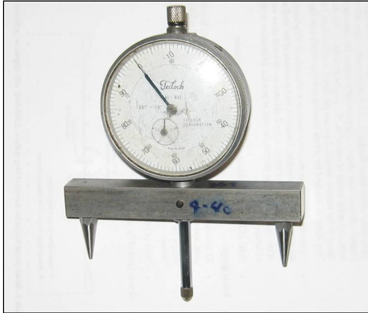
Figure 10: A small chord gauge device for measuring OOC in experimental pressure hull models (MacKay, 2007B)
