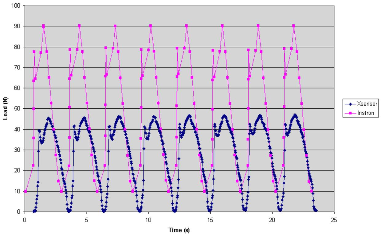
Figure 3: Cyclic Loading Results for the XSENSOR® System.
