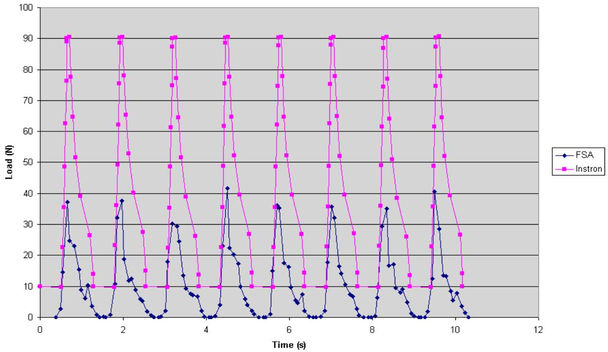
Figure 2: Cyclic Loading Results for the FSA System.
