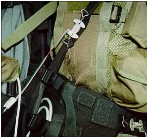
Figure 3.9 Strap Force Transducer
