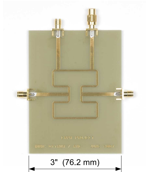
Figure 8: Fabricated Moore 1-st iteration fractal hybrid on 60-mil FR4 substrate
