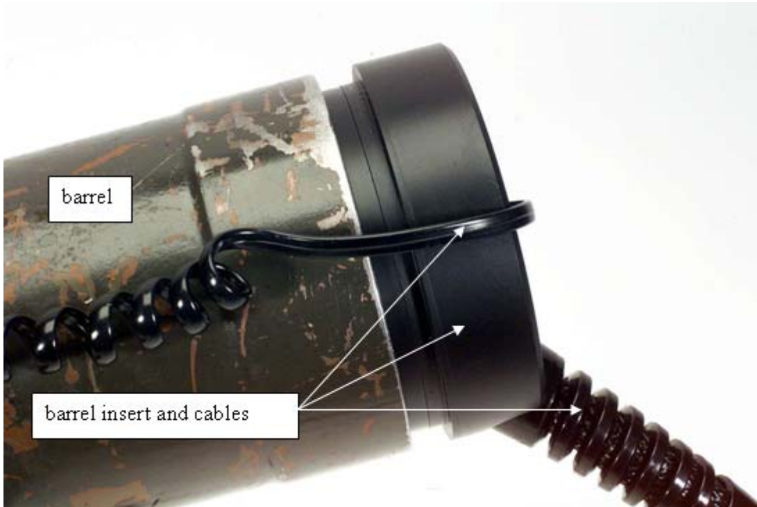
Figure 7. Barrel insert dislodged from loading a round that did not completely collapse.
