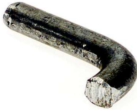
Figure 5. Improvised Sensor Latch Mount “Screw”.
