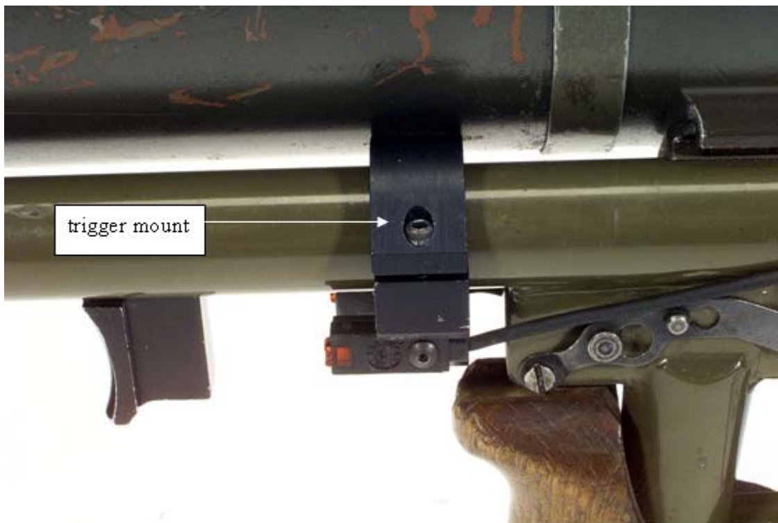
Figure 1: SAT sensor Trigger Mount correctly installed
