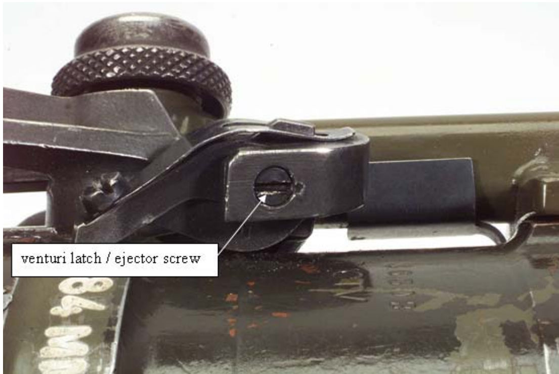
Figure 3: SRAAW(M) venturi latch / ejector screw.
