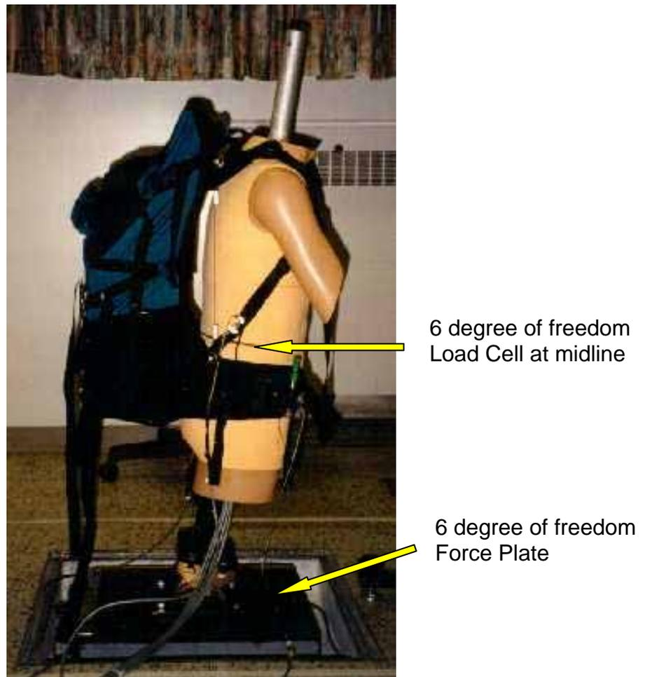
**Figure 2.** Load Distribution Tester
