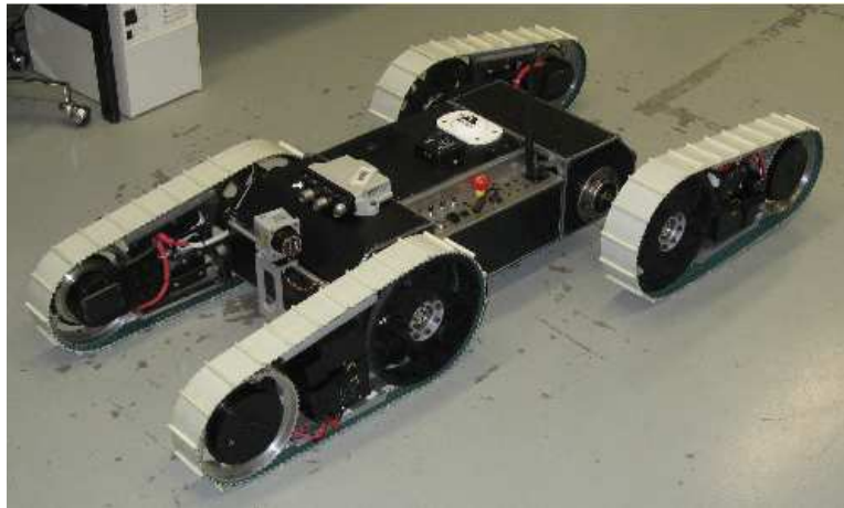
Figure 2: STRV sensors: global positioning system (GPS), inertial measurement unit (IMU) and laser range finder.
