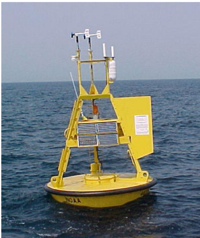
*Figure 7. A 3 meter discus buoy, the type at Station 46131 Sentry Shoal*
