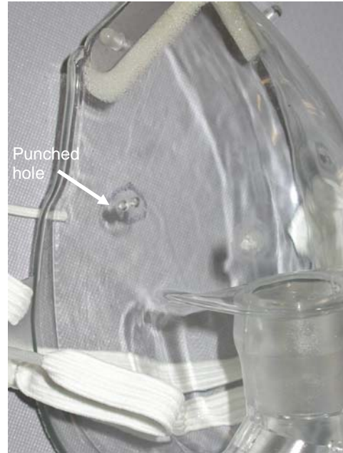
Figure 2: Holes in HiOx Mask for simulated leakage.
