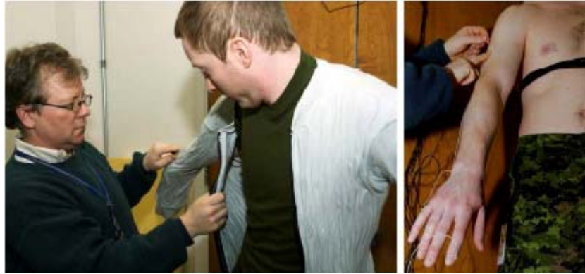
Figure 7: Views of the torso portion of the tube suit for cooling and placement of thermistors for skin temperature measurements of the finger, hand, and arm.
