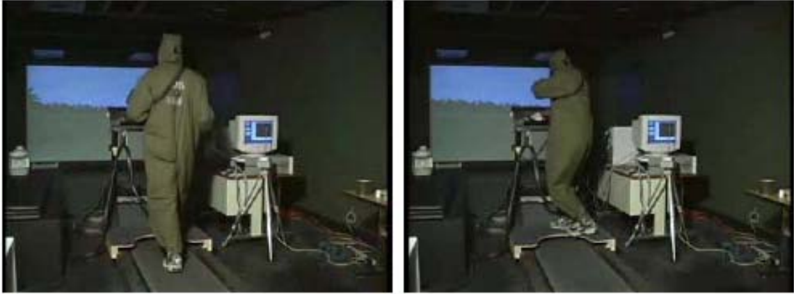
Figure 4: Experimental set-up showing the subject walking on the treadmill and dismounted on the raised platform after detecting a foe target.
