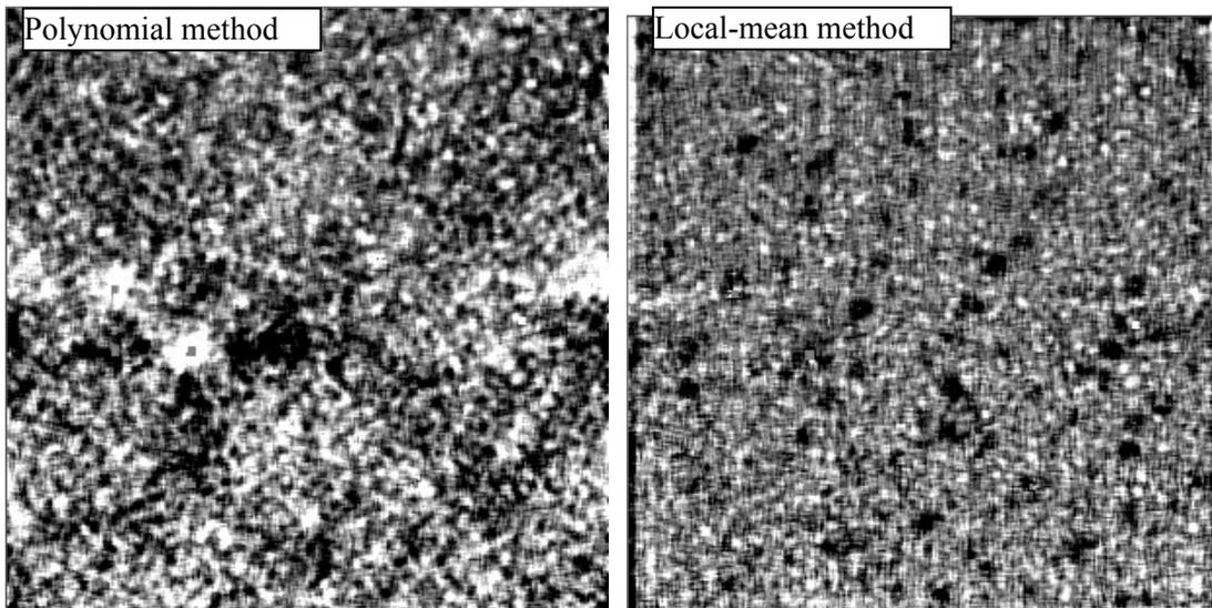
**Figure 8- Local mean of the noise calculated on the residual noise obtained by both methods. The image background is removed with the polynomial method in the left image and by the local mean in the right image.**
