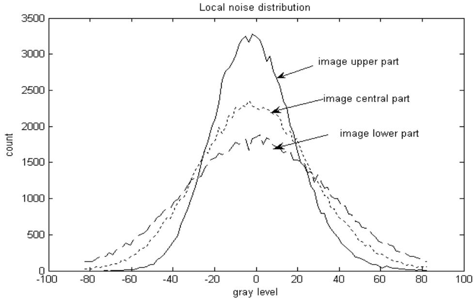
**Figure 6- Distributions of the residual noise of the image acquired in sidereal mode (in Fig. 1). Distributions are measured at the top, middle and bottom of the image. This image was acquired by the DRDC-Valcartier SofS/CD CCD camera. The noise standard deviation is more important in the bottom of the image.**
