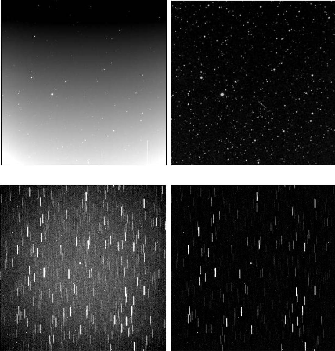
***Figure 1 – Example of image acquired in sidereal and satellite tracking mode by different CCD cameras (the background patterns are not similar). The left and right sides show the original and background corrected images.***
