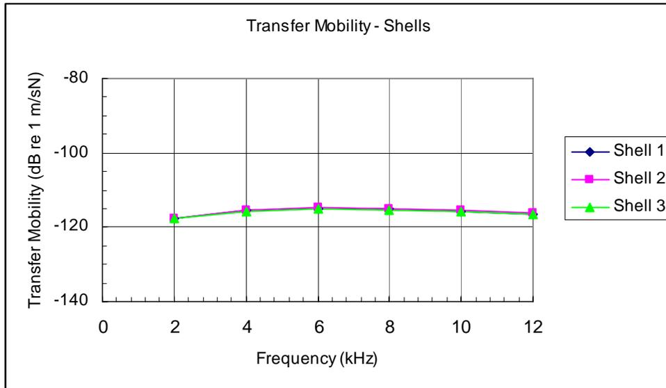
Figure 2.3 SNAP Predictions of Transfer Mobility in Shell
