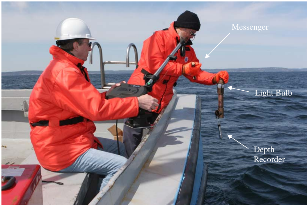
Figure 4. The authors deploying light bulbs with a “down rigger”.
