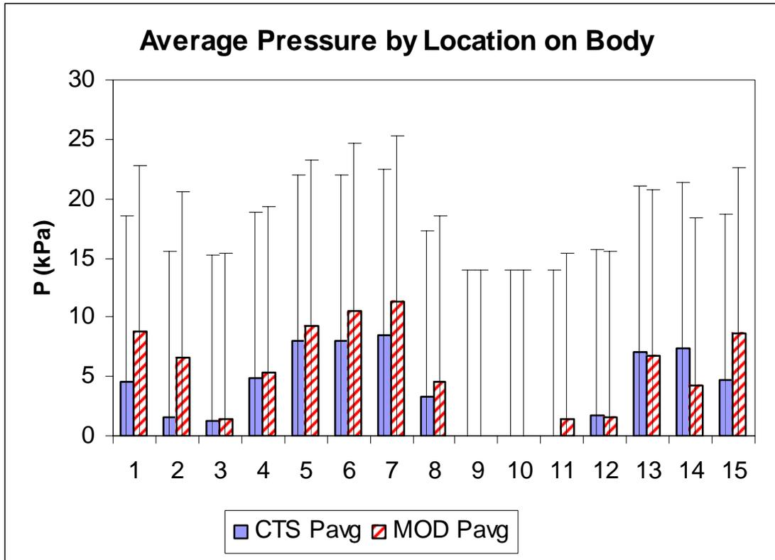
Figure 16. Average pressure on the body at all monitored sites. These values correspond to the total force experienced on each sensor location, divided by the contact area. Average pressures should typically be less than 20 kPa for continuous exposure conditions. Error bars show +/- 14 kPa which is the tested accuracy of the pressure sensors. Average pressures on sensors 9 and for both the CTS and MOD were so low as to be effectively 0. This was also the case for sensor location 11 for the CTS.
