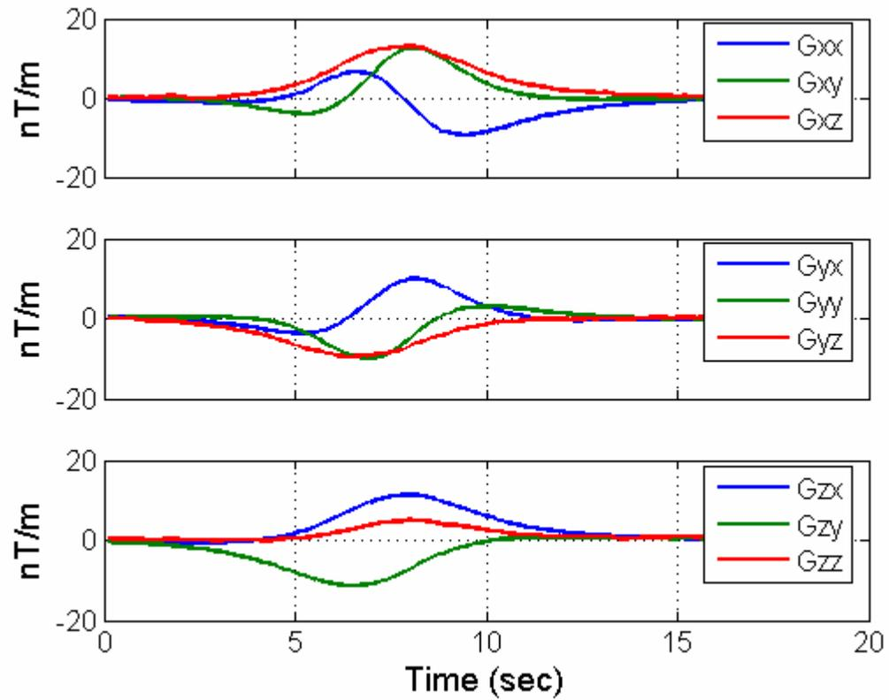
**Figure 2.** All 9 magnetic gradient components for the target on the 10m track.
