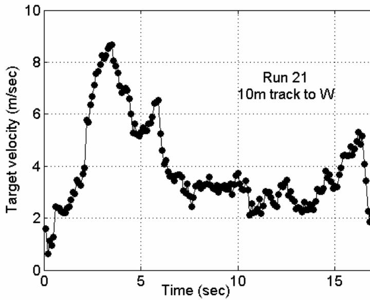
Figure 8. Estimated magnitude of target velocity (10m path).
