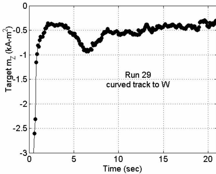
Figure 13. Estimated target Z-magnetic moment component (curved path).
