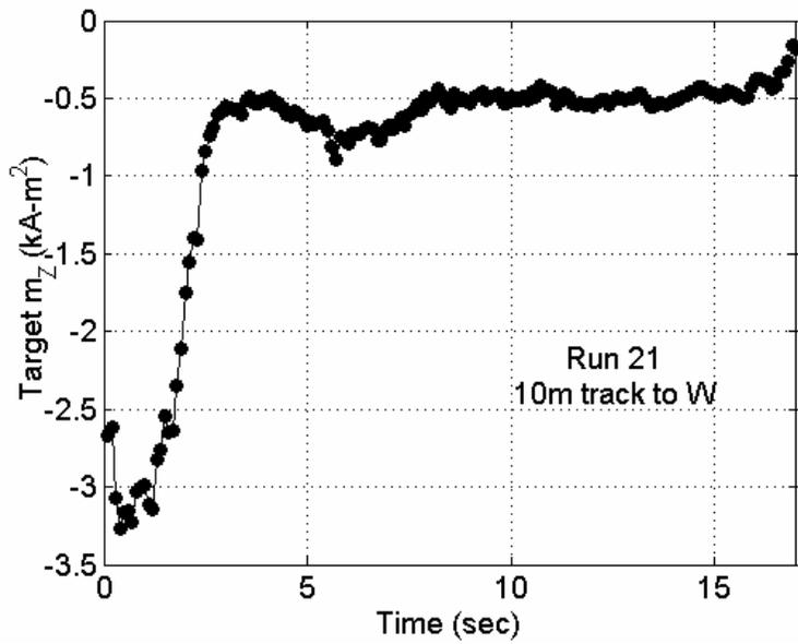
Figure 7. Estimated target Z-magnetic moment component (10m path).
