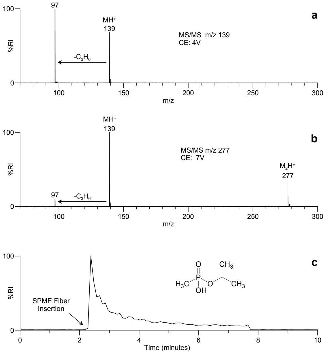
**Figure 18.** Product ion mass spectra acquired for a) isopropyl methylphosphonic acid and b) its dimer acquired during c) DESI-MS (total-ion-current: m/z 70 to 700) analysis of a SPME fiber used to sample the headspace (10 min at 40 °C) above 10 µg of isopropyl methylphosphonic acid.
