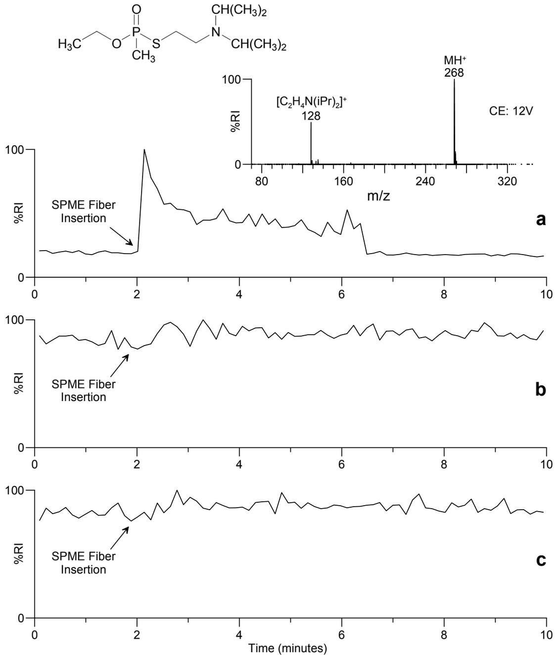
**Figure 14.** DESI-MS/MS chromatograms for  $m/z$  267 obtained during analysis of a) a SPME fiber used to sample the headspace (5 min at 80 °C) above 10  $\mu$ g of VX, b) a SPME fiber used to sample the headspace (20 min at 80 °C) above canola oil spiked at the 10  $\mu$ g/g level with VX and c) a SPME fiber used to sample the headspace (10 min at 80 °C) above corn meal spiked at the 10  $\mu$ g/g level with VX. Inset: typical product ion mass spectrum for VX.
