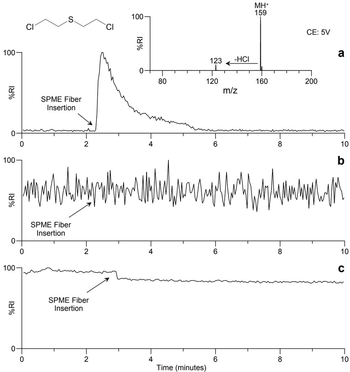
**Figure 15.** DESI-MS/MS chromatograms for  $m/z$  159 obtained during analysis of a) a SPME fiber used to sample the headspace (10 min at 40 °C) above 10 µg of mustard (H), b) a SPME fiber used to sample the headspace (10 min at 40 °C) above canola oil spiked at the 10 µg/g level with H and c) a SPME fiber used to sample the headspace (10 min at 40 °C) above corn meal spiked at the 10 µg/g level with H. Inset: typical product ion mass spectrum for H.
