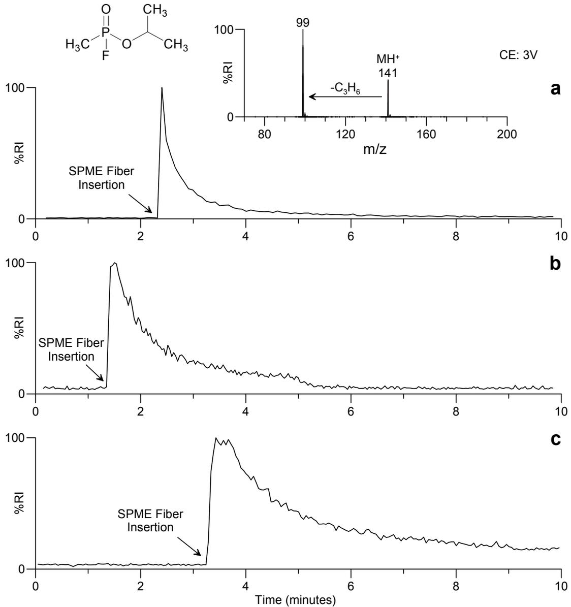
**Figure 10.** DESI-MS/MS chromatograms for  $m/z$  141 obtained during analysis of a) a SPME fiber used to sample the headspace (15 s at 40 °C) above 5  $\mu$ g of sarin (GB), b) a SPME fiber used to sample the headspace (10 min at 40 °C) above canola oil spiked at the 5  $\mu$ g/g level with GB and c) a SPME fiber used to sample the headspace (10 min at 40 °C) above corn meal spiked at the 5  $\mu$ g/g level with GB. Inset: typical product ion mass spectrum for GB.
