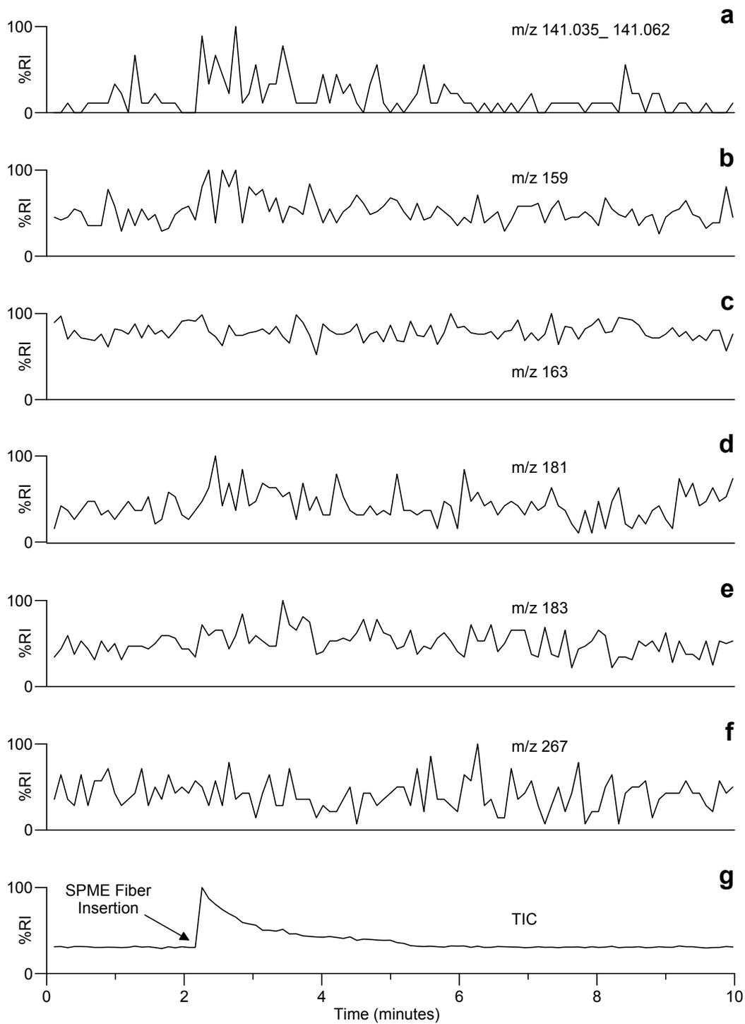
**Figure 5.** DESI-MS analysis of a SPME fiber used to sample the headspace (20 min at 80 °C) above a canola oil blank. Reconstructed-ion-current chromatograms for a) m/z 141 (window narrowed to exclude a background ion of the same nominal mass as sarin), b) m/z 159, c) m/z 163, d) m/z 181, e) m/z 183 and f) m/z 267. g) Total-ion-current (m/z 70 to 700) chromatogram.
