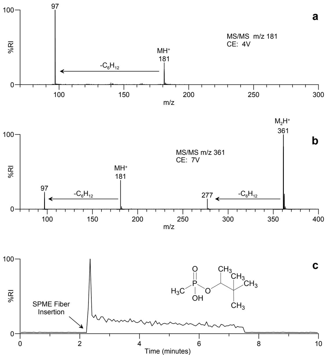
**Figure 19.** Product ion mass spectra acquired for a) pinacolyl methylphosphonic acid and b) its dimer acquired during c) DESI-MS (total-ion-current: m/z 70 to 700) analysis of a SPME fiber used to sample the headspace (10 min at 80 °C) above 10 μg of pinacolyl methylphosphonic acid.
