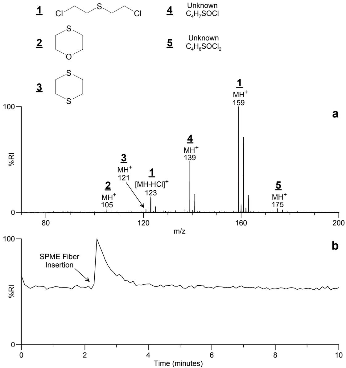
**Figure 17.** a) ESI-MS data acquired during DESI-MS analysis of a SPME fiber used to sample the headspace (10 min at 40 °C) above 40  $\mu$ g of a munitions grade mustard sample, HQ. Mustard (H) and four related compounds were detected. Sesquimustard (Q) was not detected. b) DESI-MS total-ion current ( $m/z$  70 to 700) chromatogram obtained during this analysis.
