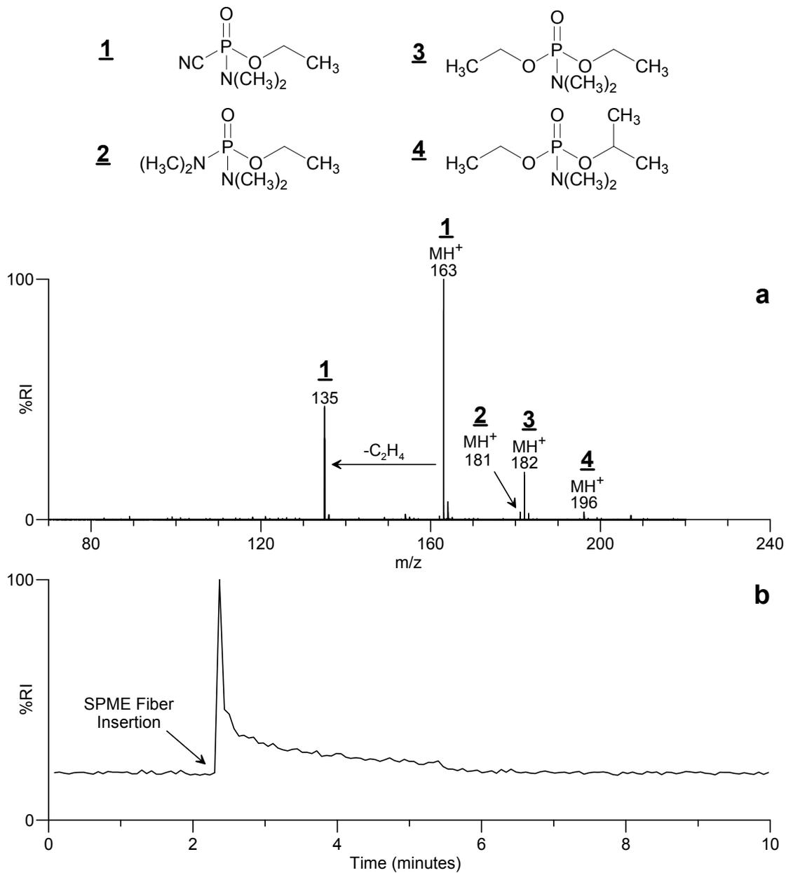
**Figure 16.** a) ESI-MS data acquired during DESI-MS analysis of a SPME fiber used to sample the headspace (10 min at 40 °C) above canola oil spiked at the 20 µg/g level with a munitions grade sample of tabun (GA). Tabun and three related compounds were detected. b) DESI-MS total-ion current (m/z 70 to 700) chromatogram obtained during this analysis.
