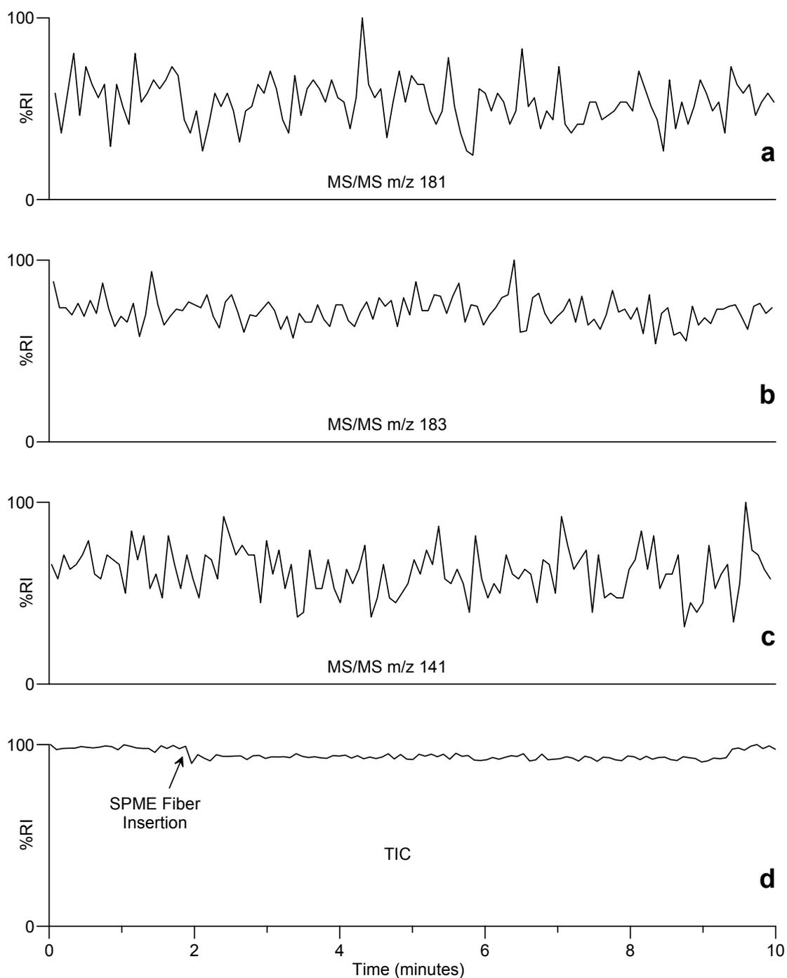
**Figure 4.** DESI-MS and MS/MS analysis of a SPME fiber used to sample bottled water blank. The SPME fiber was inserted into the water for 2 min at ambient temperature. Product ion chromatograms acquired for a) m/z 181, b) m/z 183 and c) m/z 141. d) Total-ion-current (m/z 70 to 700) chromatogram obtained during the same analysis.
