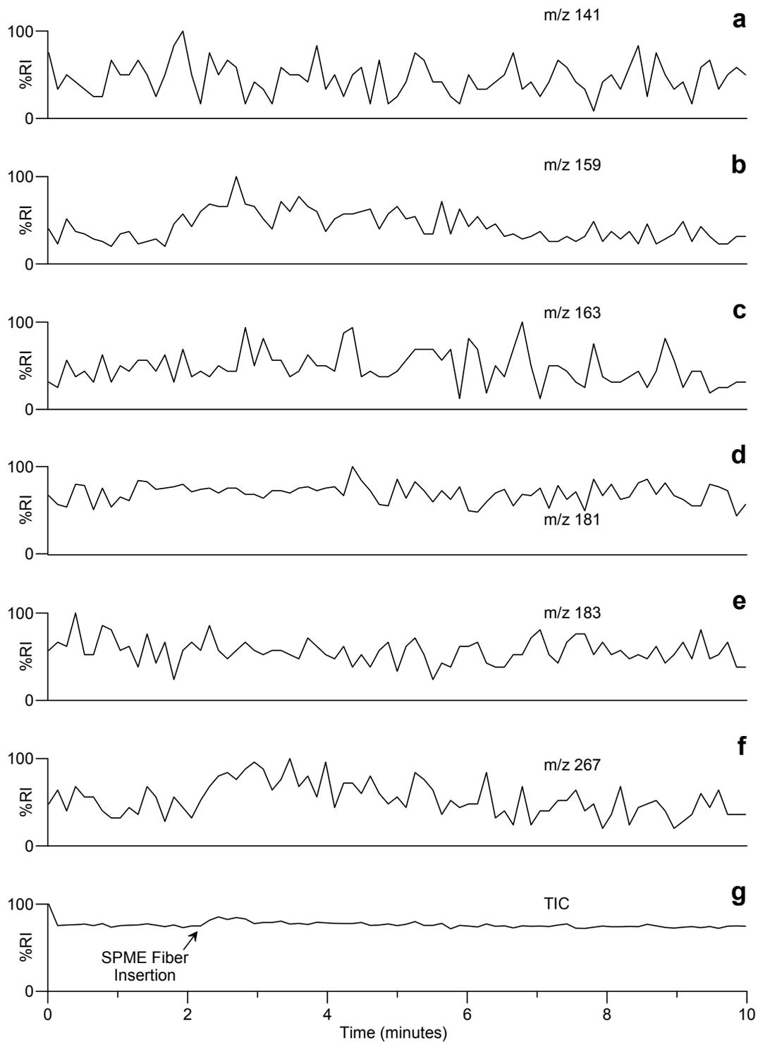
**Figure 7.** DESI-MS analysis of a SPME fiber used to sample the headspace (5 min at 80 °C) above a corn meal blank. Reconstructed-ion-current chromatograms for a)  $m/z$  141, b)  $m/z$  159, c)  $m/z$  163, d)  $m/z$  181, e)  $m/z$  183 and f)  $m/z$  267. g) Total-ion-current ( $m/z$  70 to 700) chromatogram.
