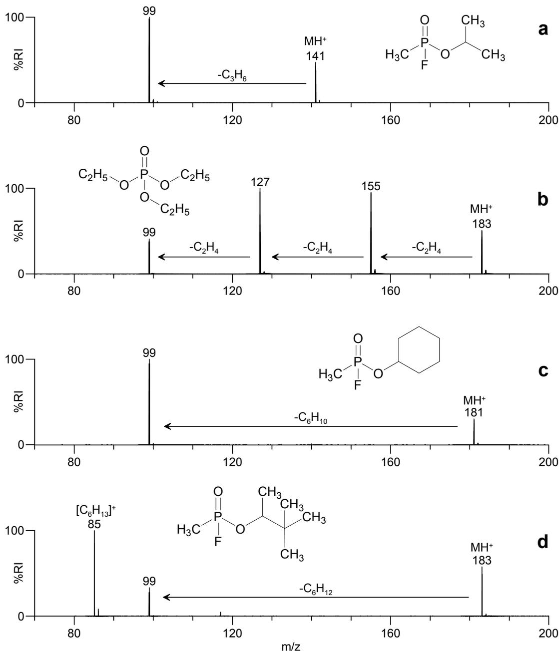
**Figure 2.** Product ion mass spectra acquired for a) sarin (CE: 3V), b) triethyl phosphate (CE: 10V), c) cyclohexyl methylphosphonofluoridate (CE: 4V) and d) soman (CE: 3V) during LC-ESI-MS/MS analysis of a bottle water sample spiked at the 10  $\mu\text{g}/\text{mL}$  level with these four compounds.
