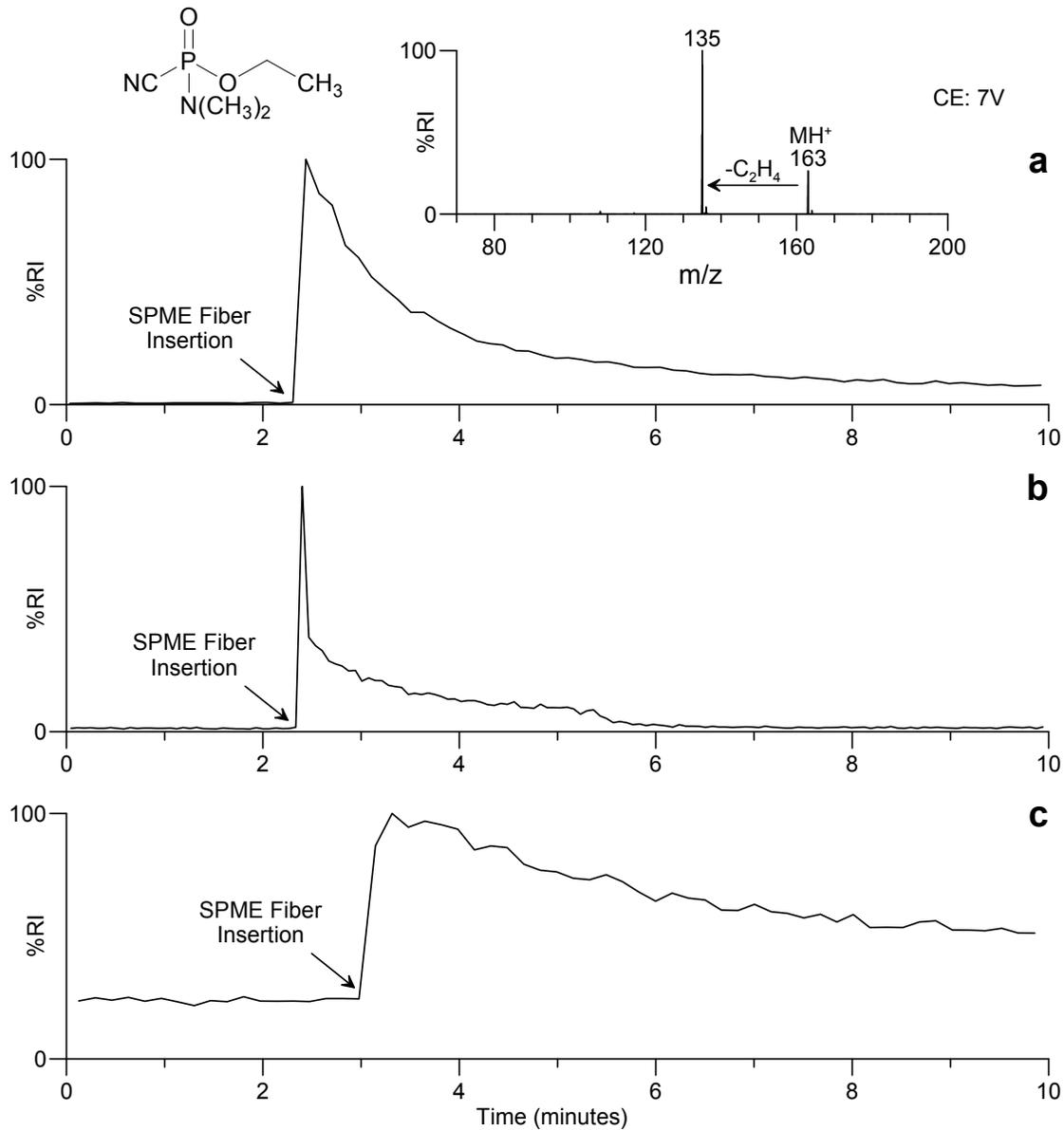
**Figure 11.** DESI-MS/MS chromatograms for  $m/z$  163 obtained during analysis of a) a SPME fiber used to sample the headspace (2 min at 40 °C) above 0.5 µg of tabun (GA), b) a SPME fiber used to sample the headspace (10 min at 40 °C) above canola oil spiked at the 15 µg/g level with GA and c) a SPME fiber used to sample the headspace (10 min at 40 °C) above corn meal spiked at the 15 µg/g level with GA. Inset: typical product ion mass spectrum for GA.
