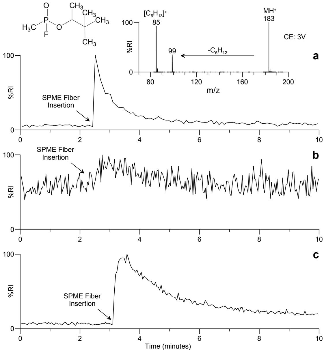
**Figure 12.** DESI-MS/MS chromatograms for  $m/z$  183 obtained during analysis of a) a SPME fiber used to sample the headspace (15 s at 40 °C) above 5  $\mu$ g of soman (GD), b) a SPME fiber used to sample the headspace (10 min at 40 °C) above canola oil spiked at the 10  $\mu$ g/g level with GD and c) a SPME fiber used to sample the headspace (10 min at 40 °C) above corn meal spiked at the 10  $\mu$ g/g level with GD. Inset: typical product ion mass spectrum for GD.
