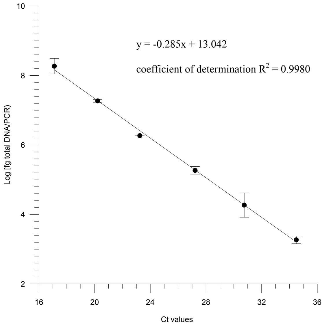
**Figure 2. Standard Curve for the *lef* Assay using *B. anthracis* Ames total DNA in solution**
