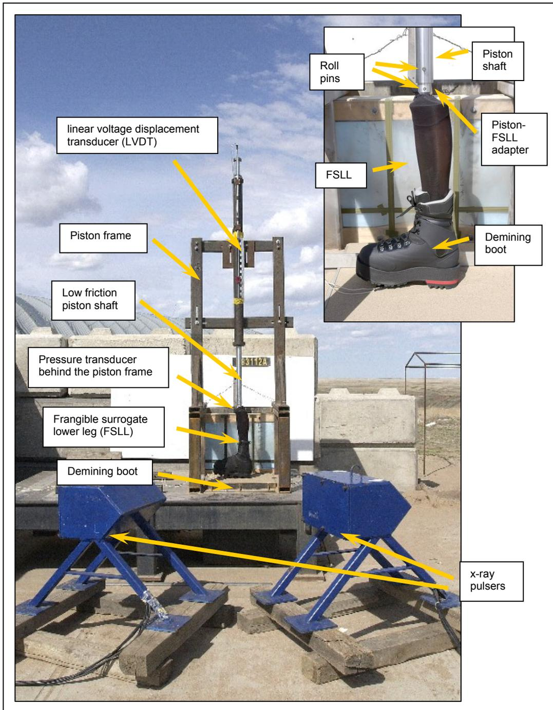
**Figure 2. Piston shaft apparatus**
