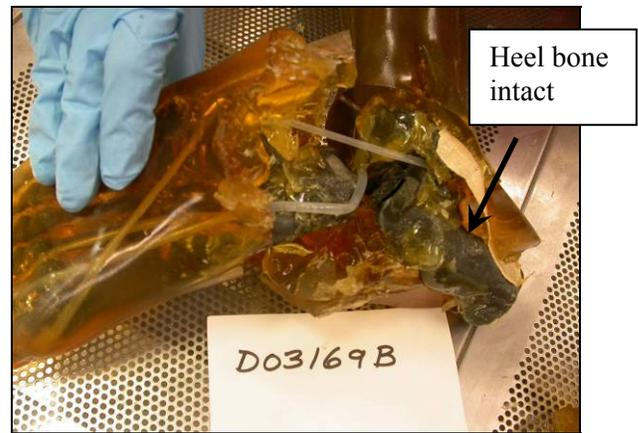
**Figure 3b.** This boot used for this specimen was effective against 25g of C4. (Note the bones and tendons are intact)
