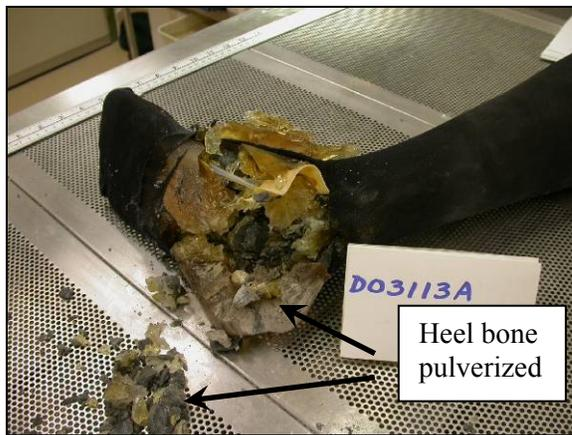
**Figure 3a.** The boot used for this specimen was NOT effective against 75g of C4. (Note the pieces of the shattered heel bone)
