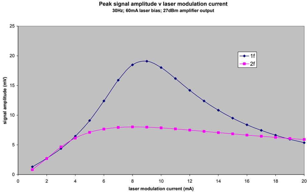
**Figure 5. Variation of acoustic signals with laser modulation current**
