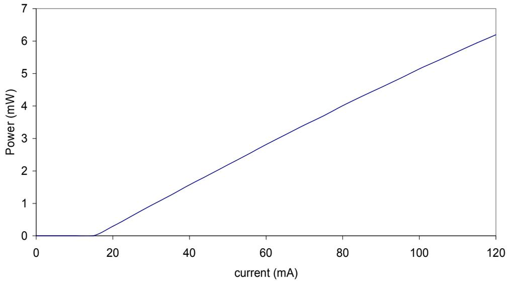
**Figure 3. DFB Laser characteristics**
