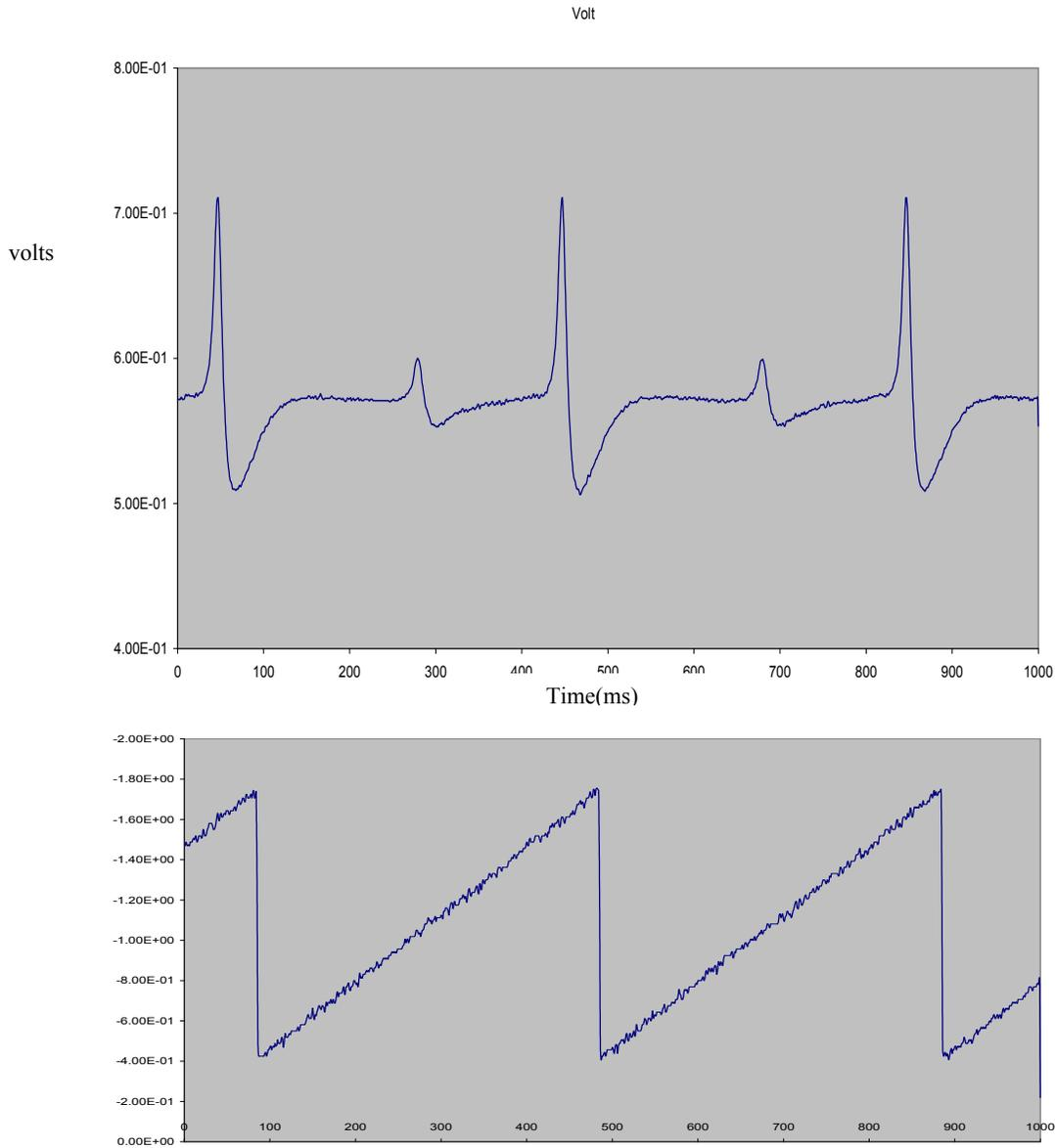
**Figure 10. Acoustic signal (upper trace) generated as a result of ramping the laser drive current (lower trace)**
