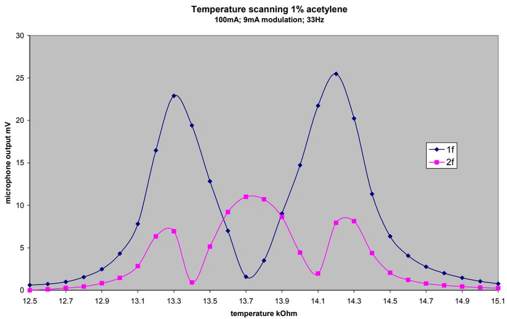
**Figure 7. Temperature scanning with laser bias current of 100mA**
