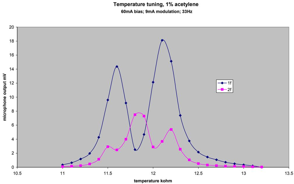
**Figure 6. Temperature scanning with laser bias current of 60mA**
