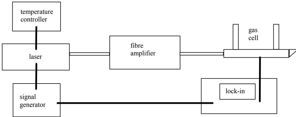
**Figure 1. Gas cell interrogation system**
