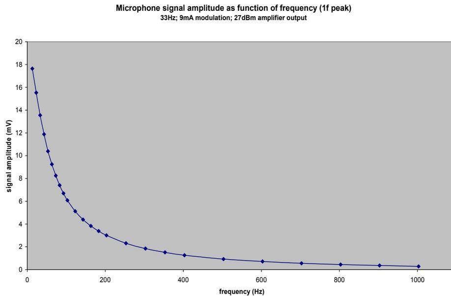
**Figure 8. Variation of signal amplitude with modulation frequency**
