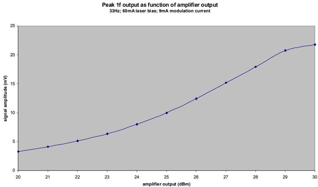
*Figure 9. Variation of acoustic signal amplitude with amplifier output*
