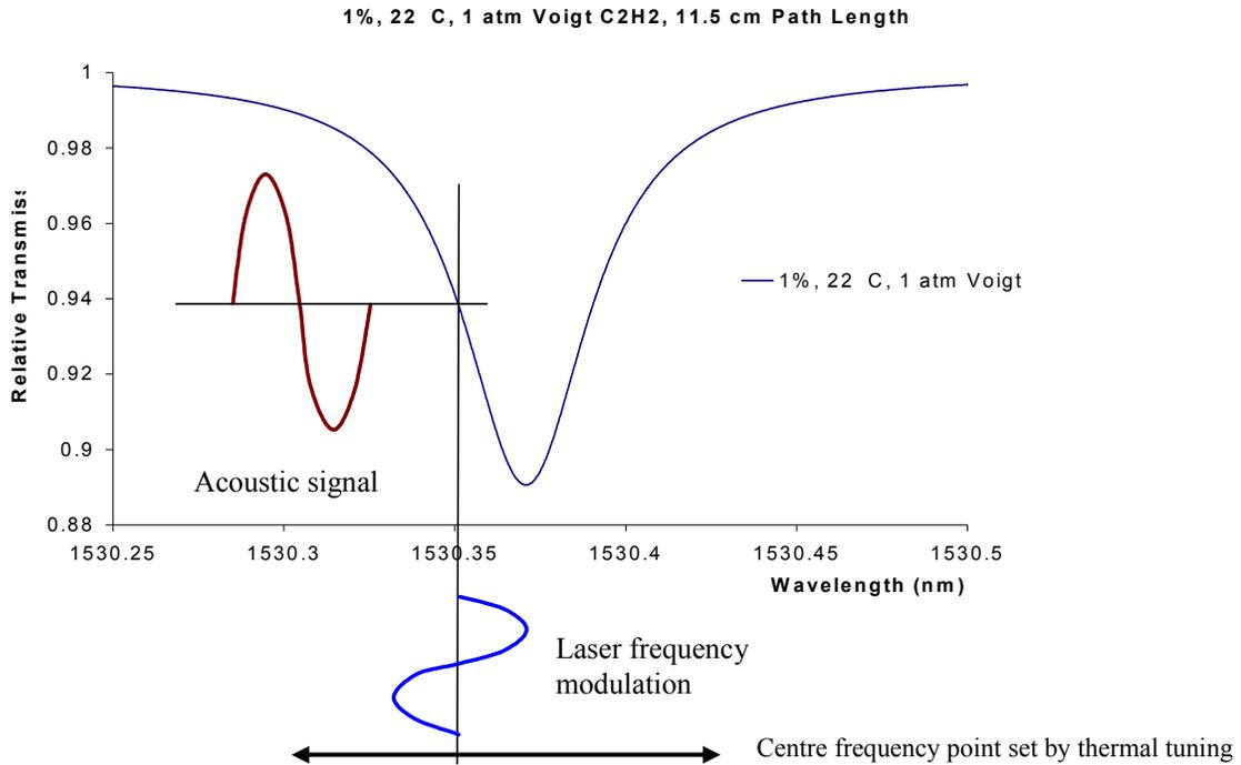
**Figure 4. Generation of an acoustic signal through laser frequency modulation**
