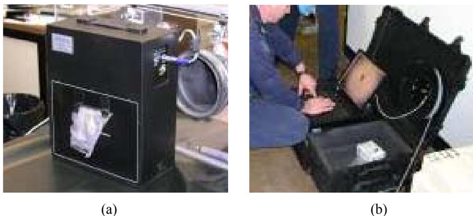
**Figure 4.** Explosives detection using foXray machine. (a) Radiography unit and (b) Visual display.
