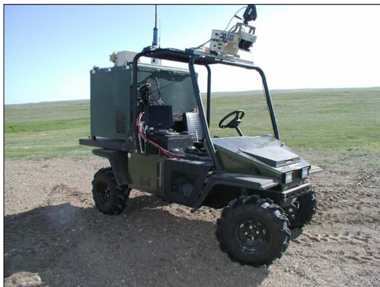
Figure 2: One of two modified Koyker Raptors used in DRDC's ALS Project. Each Raptor used one or more roof mounted SICK lasers and stereo cameras; Differential GPS and IMU; and wireless mesh networking routers.
