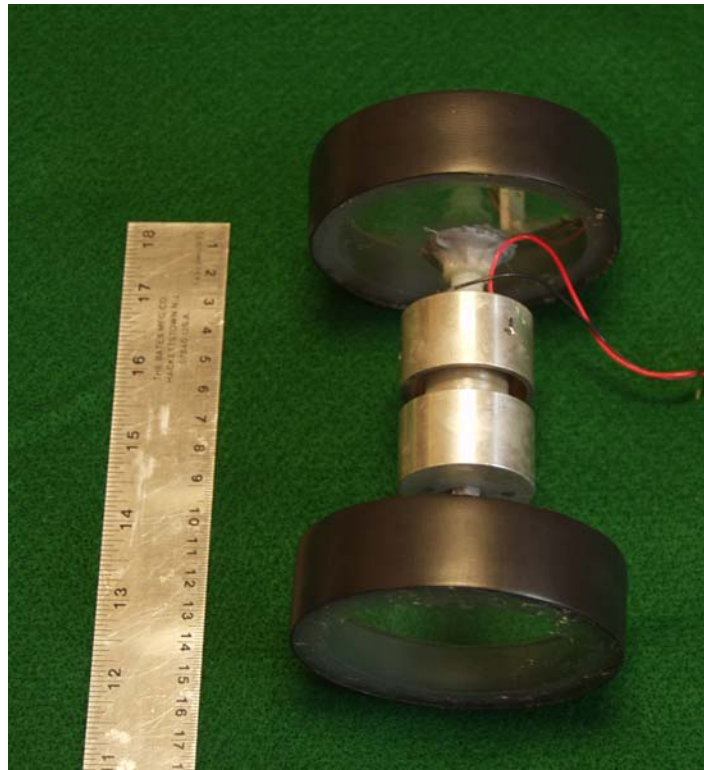
Figure 8. HF MMPP with prototype rigid air-cavity attenuators.
