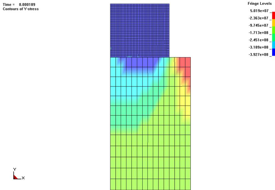
**Figure 5.** Radial stress contours with less elements in region I ( $V_{striker} = 17.3$  m/s)
