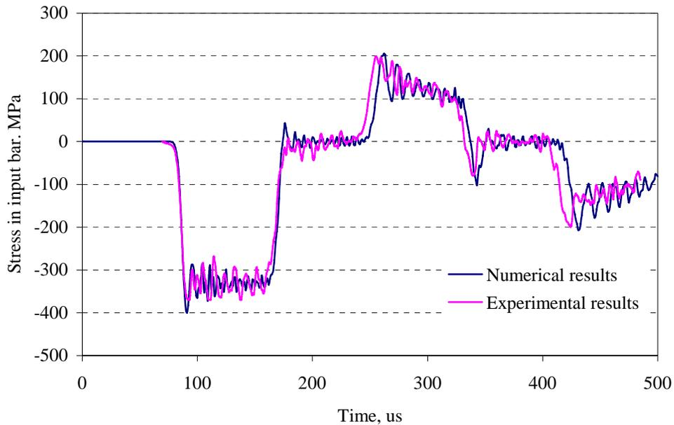
**Figure 9.** Comparison between experimental and numerical results for the incident bar ( $D_{\text{sample}}=10.5 \text{ mm}$ ,  $L_{\text{sample}}=5 \text{ mm}$ ,  $V_{\text{striker}}=17.3 \text{ m/s}$ )
