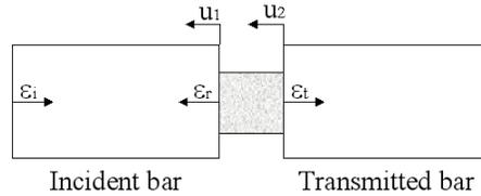
**Figure 2.** Expanded view of incident bar, specimen and transmitted bar
