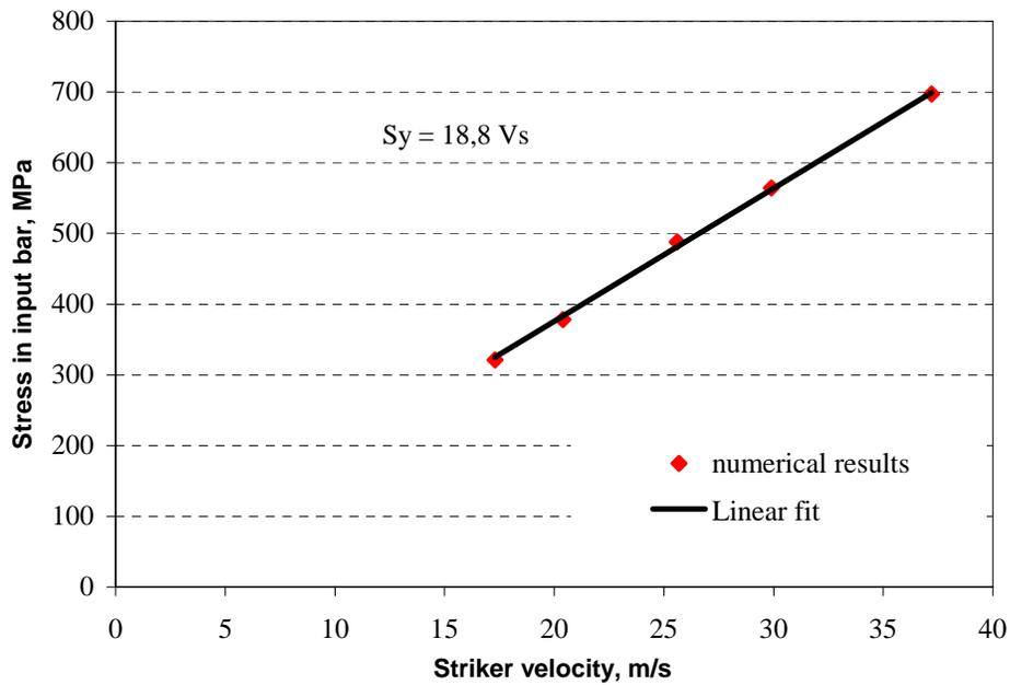
**Figure 11.** Linear relationship between striker velocity and stress in the incident bar
