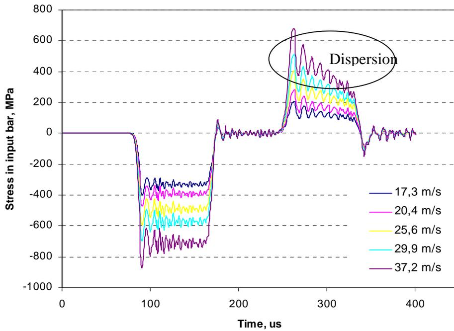
**Figure 10.** Effect of striker velocity on the stress generated in the incident bar
