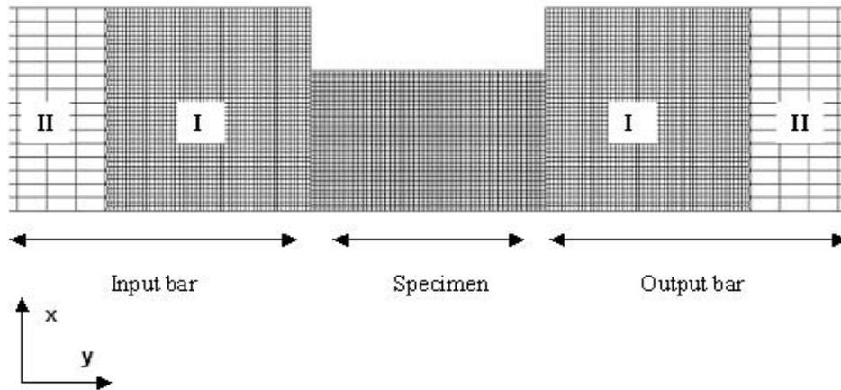
*Figure 4. Typical finite elements mesh used for simulation*
