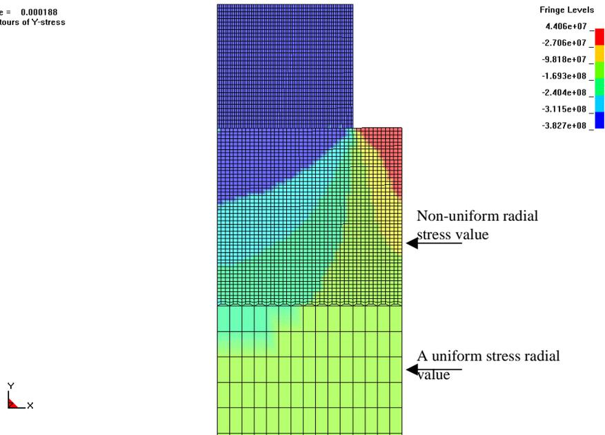
**Figure 6.** Radial stress contours with fine elements in region I ( $V_{striker} = 17.3$  m/s)
