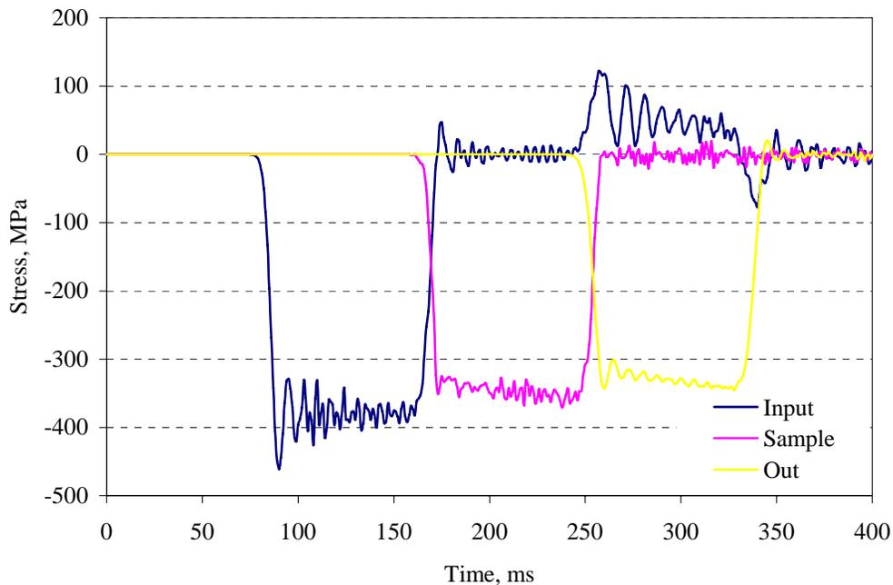
**Figure 8.** Incident and transmitted radial stress ( $D_{\text{sample}}=10.5$  mm,  $L_{\text{sample}}=5$  mm,  $V_{\text{striker}}=35.5$  m/s)
