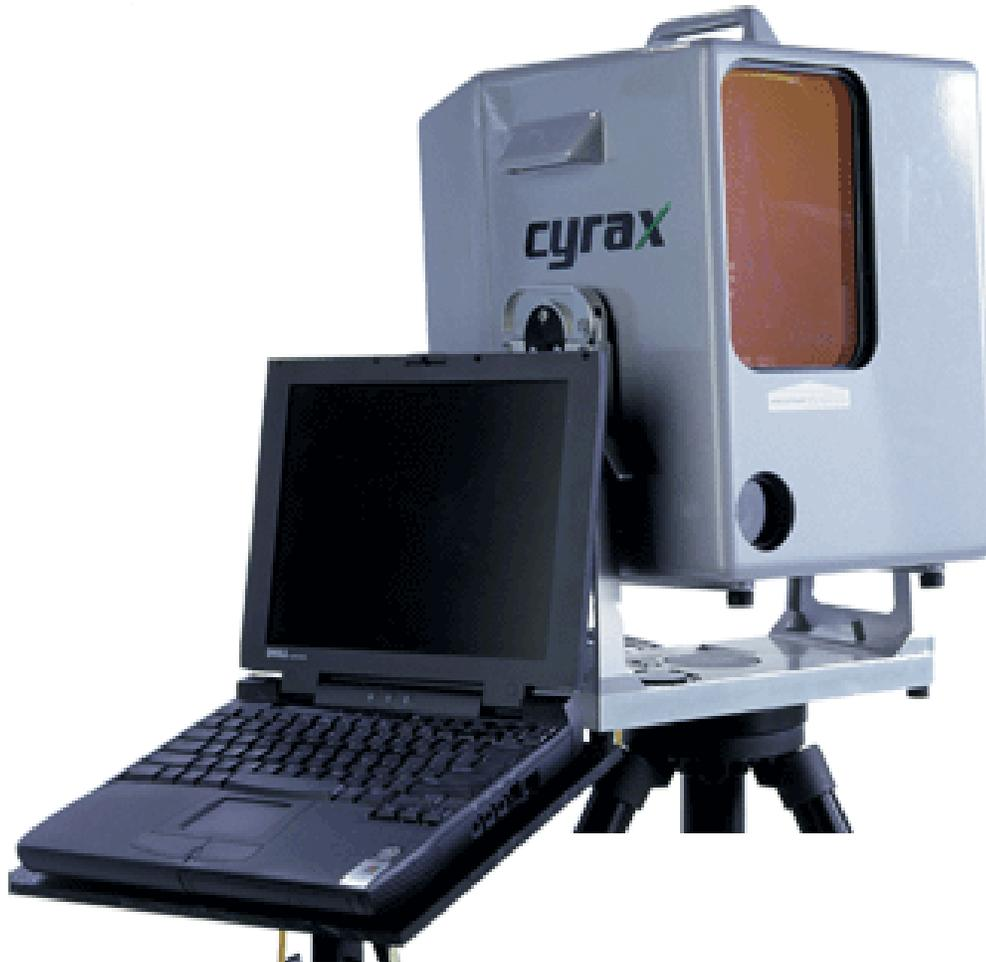
*Figure 2. Cyrax 2500 Laser Scanner and Controller*
