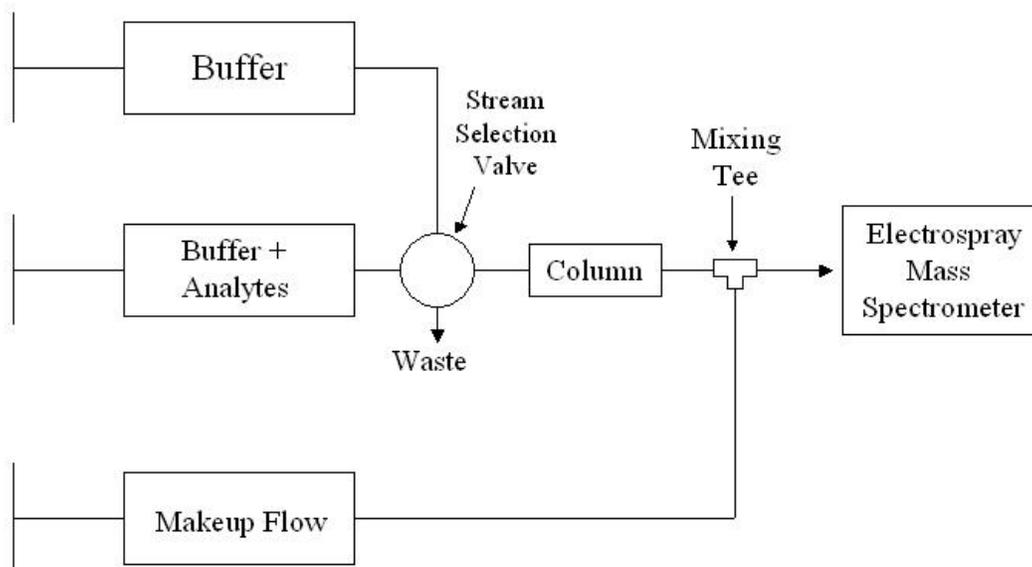
**Figure 4.** Schematic of the FAC-MS system for monitoring molecular interactions. Syringes containing either buffer or buffer containing analytes (ligands) are connected to the FAC column through a stream selection valve. Makeup flow, typically a volatile, organic solvent, is introduced immediately postcolumn through a mixing tee, with the combined flow introduced into an electrospray mass spectrometer.
